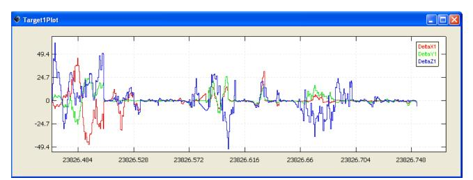
Figure 4. Tracking results of EKF (where DeltaX1, DeltaY1, and DeltaZ1 are the tracking in X-axis, Y-axis, and Z-axis, respectively)
