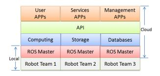
Fig. 2. Abstract Architecture of a Cloud Robotics System
