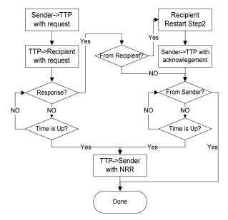
Figure 3. Flowchart of Resolve mode.
