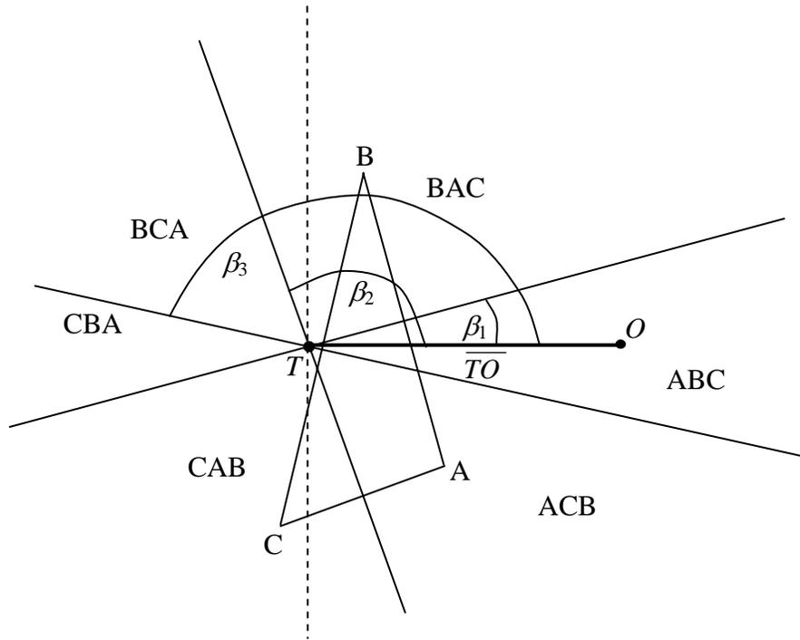
Figure A-1. The four parameters  $\overline{TO}$ ,  $\beta_1$ ,  $\beta_2$ , and  $\beta_3$  that define a spatial model observation.
