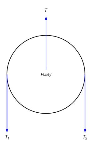
In the above figure, we assume that the mass of pulley is zero. The pulley is at rest. Then we have
