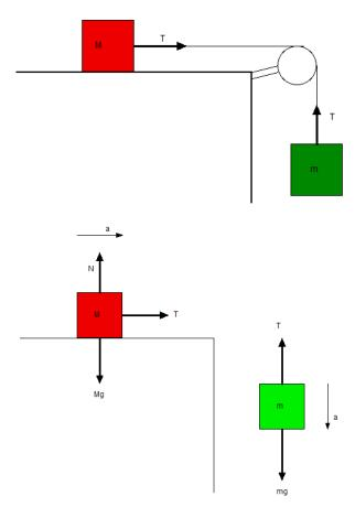
We apply the Newton's second law to free body diagrams (in this case the masses m and M)
