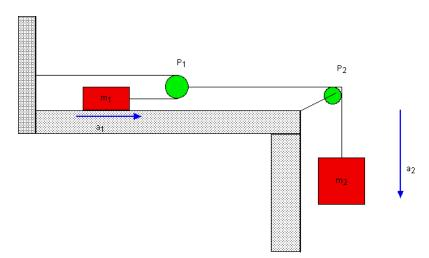
Suppose that the positions of P<sub>1</sub> and mass  $m_1$  are expressed by  $x_p$  and  $x_1$ . The length of the string through the pulley P<sub>1</sub> is
