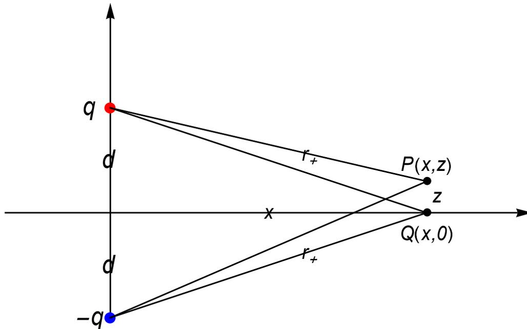
Here we find the electric potential at the point  $P(x, z)$  due to the electric dipole moment with  $p = 2qd$ . We also find the expression of the electric field at the point  $Q(x, 0)$ .
