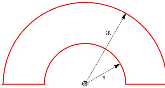
A rod with uniform linear charge density  $\lambda$  is bent into the shape above. Find the potential at the center for this configuration. We use the above results. Then we have
