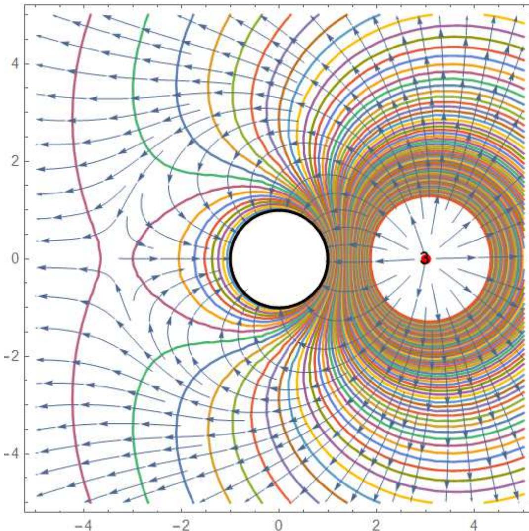
**Fig.** Electric field lines for  $a = 1$ ,  $b = 3$ ,  $q = 3$ , and  $q' = -q(a/b) = -1$ . The zero-equipotential surface exists as a sphere of radius 1 centered at  $x = 0$  and  $y = 0$ . The charge of ( $q = 3$ ) and the charge ( $q' = -1$ ) are located at  $x = 1/3$  and  $x = 3$ , respectively.
