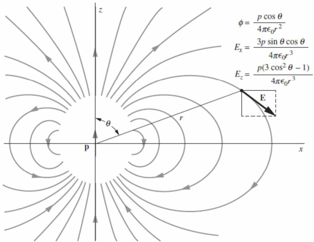
**Fig.** Electric field due to an electric dipole moment (Purcell and Morin). E.M. Purcell and D.J. Morin, *Electricity and Magnetism*, 3<sup>rd</sup> edition (Cambridge, 2013).
