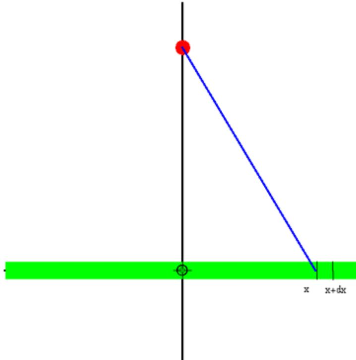
A total charge  $Q$  is distributed uniformly along a straight rod of length  $L$ . Find the potential at point P at a distance  $h$  from the midpoint of the rod. The potential at P due to a small segment of the rod, with length  $dx$  and charge  $dQ$ , located at the position is given by
