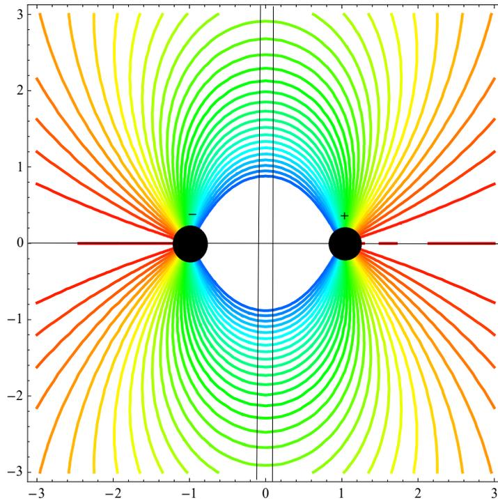
We consider a point on the conducting sheet at the distance  $\rho$  from the point directly beneath the positive charge. The electric field at this point is normally to the surface and is directed into it. The electric field resulting from both the positive point charge and the negative point charge is normal to the sheet and is given by
