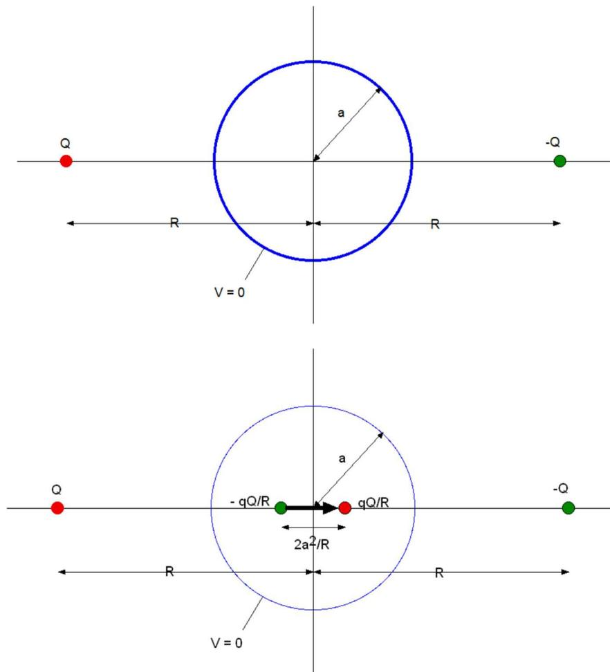
How does the electric field change when the conducting sphere (radius  $a$ ) is put in the uniform electric field  $\mathbf{E}_0$  along the  $x$  axis. Suppose that this electric field is generated by two point charges of  $Q$  at  $x = -R$  and  $-Q$  at  $x = R$ . The electric field at the sphere is  $2Q/(4\pi\epsilon_0 R^2)$ . In the limit of  $R \rightarrow 0$ , the field is parallel to the  $x$  axis.
