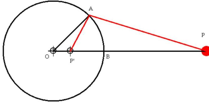
**Fig.** The point charge  $q$  induces charges on a grounded conducting sphere whose fields are those of an image charge  $q'$  placed at the point shown.  $AP = r_1$ ,  $P'A = r_2$ ,  $OA = a$ ,  $OP = b$ ,  $OP' = a^2/b$ ,  $q' = (-a/b)q$ . We choose  $b = 3$ ,  $a = 1$ ,  $q = 3$ ,  $q' = -1$ .  $OP' = 1/3$ ,  $OA = 1$ ,  $OP = 3$  in the above figure (using Mathematica).
