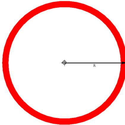
A spherical shell of radius  $R$  carries charge  $Q$  uniformly distributed over the surface. Determine  $V$  inside and outside. For  $r > R$ , we have  $V = \frac{1}{4\pi\epsilon_0} \frac{Q}{r}$ . For  $r < R$ , there is no charge.
