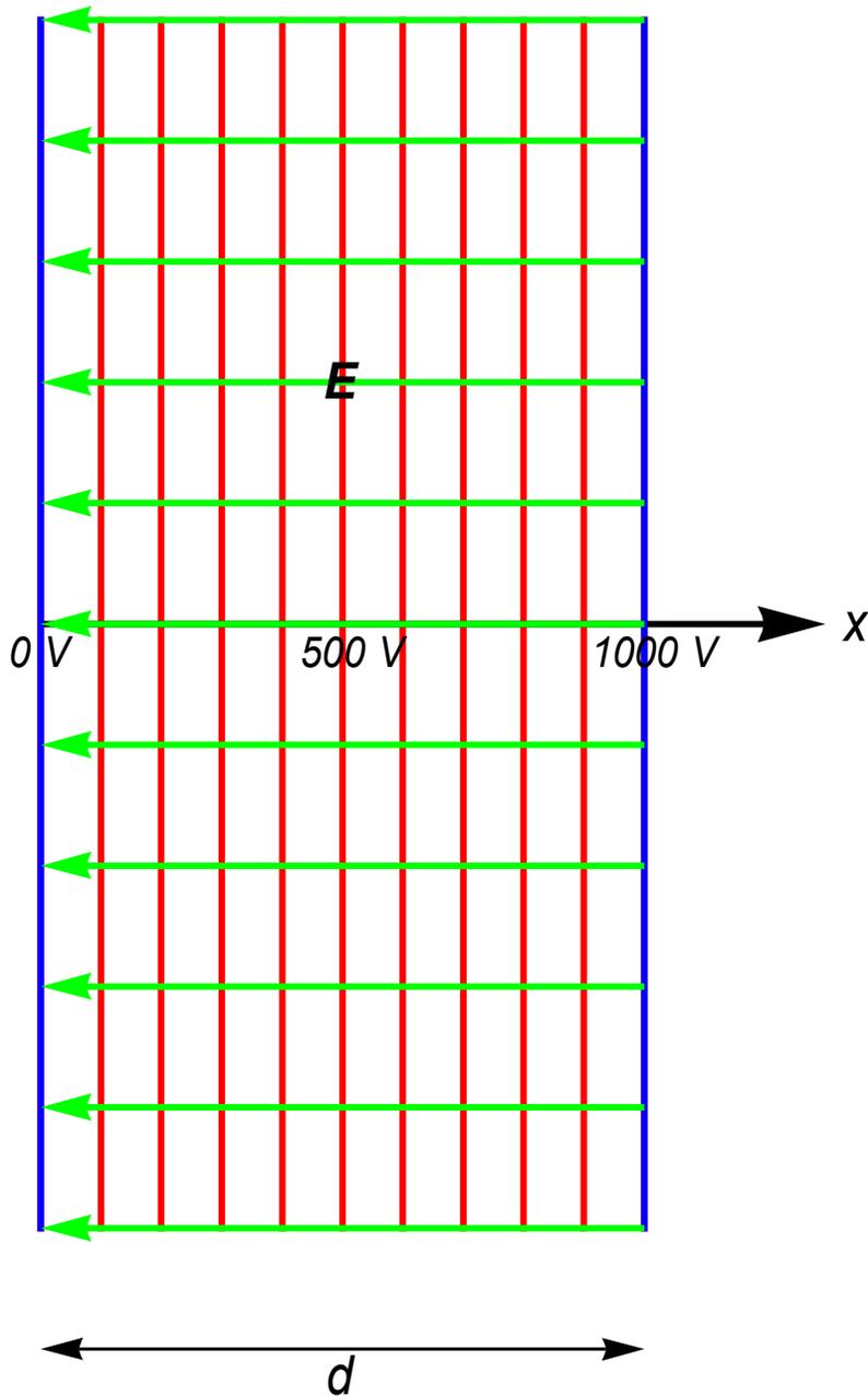
The direction of the electric field (denoted by the green line) is along the negative direction. The red line denotes the constant  $V$  with  $V = 0 - 1000 \text{ V}$ . The equipotential line with the constant  $V$  is perpendicular to the electric field  $E$ .
