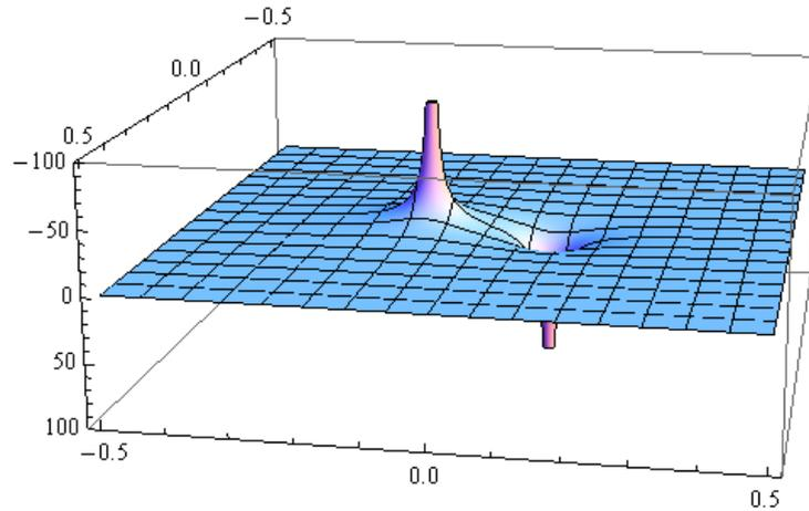
The electric potential at a point  $P$  in space due to two, or more point charges is obtained from the superposition principle.
