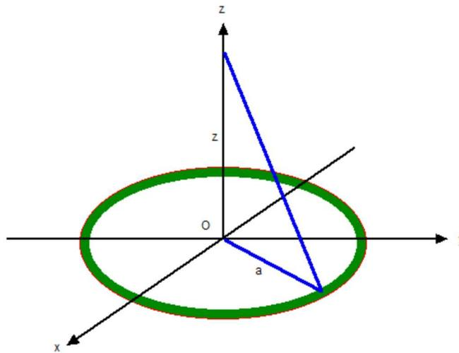
Charge  $Q$  is uniformly distributed on a ring of radius  $a$ . Determine the electric potential at a point on the axis of the ring a distance  $z$  from the center.
