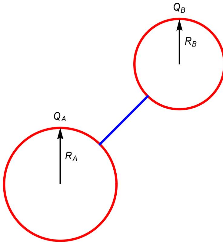
**Fig.2** The field of a pointed object can be approximated by that of two spheres at the same potential.
