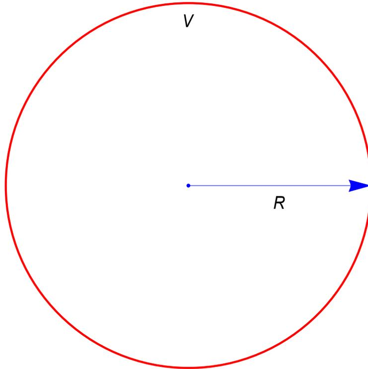
**Fig.** Schematic diagram of the van de Graaff.  $R = 0.3$  m.  $C = 33.4$  pF. The standard value of air dielectric breakdown is  $3\text{kV/mm} = 3000$  kV/m =  $3\text{MV/m}$ ).
