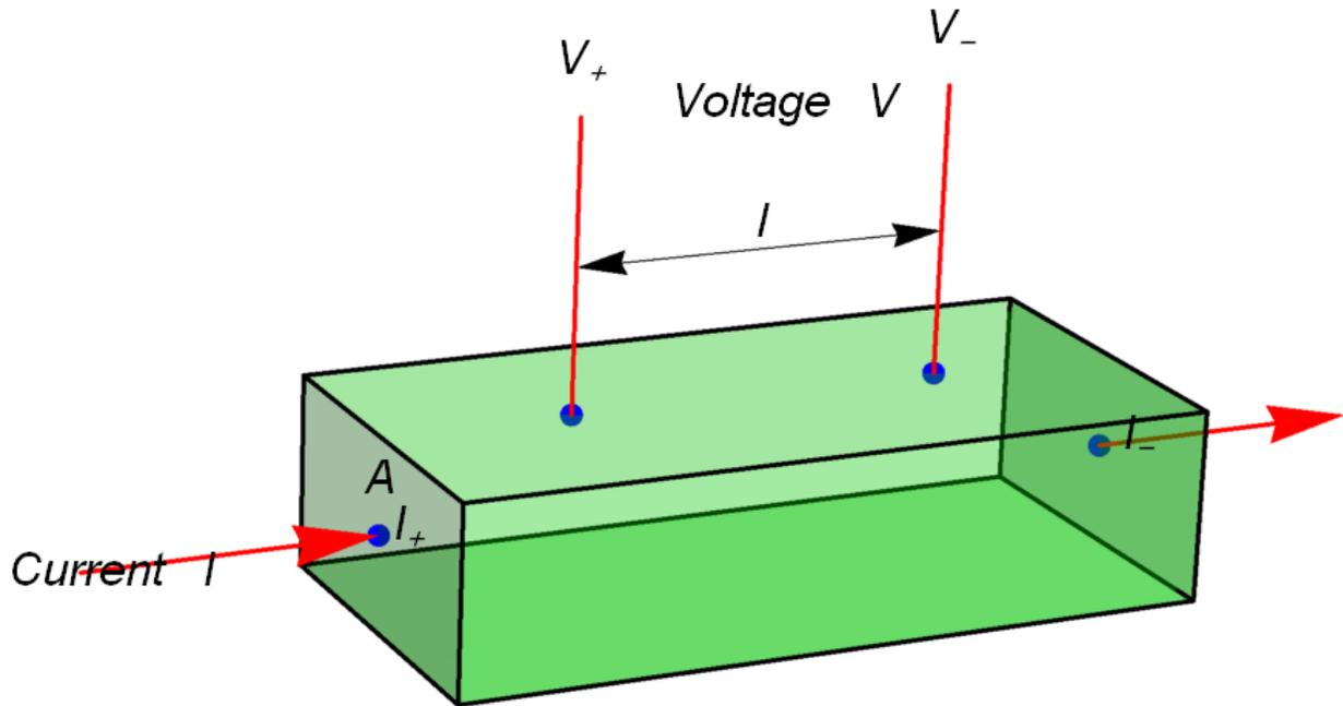
**Fig.1** Four probes measurement of electrical resistivity of metal. The cross-sectional area is  $A$ . Two current probes ( $I_+$ ,  $I_-$ ). Two voltage probes ( $V_+$ ,  $V_-$ ).  $l$  is the distance between two voltage probes. The current is fed to one of the current probe ( $I_+$ ) using constant current source. The voltage between the voltage probes can be measured using a digital nano-voltmeter.
