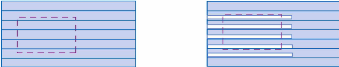
Fig.3 Eddy currents can be reduced by (a) laminating the slab, or (b) making cuts on the slab.
