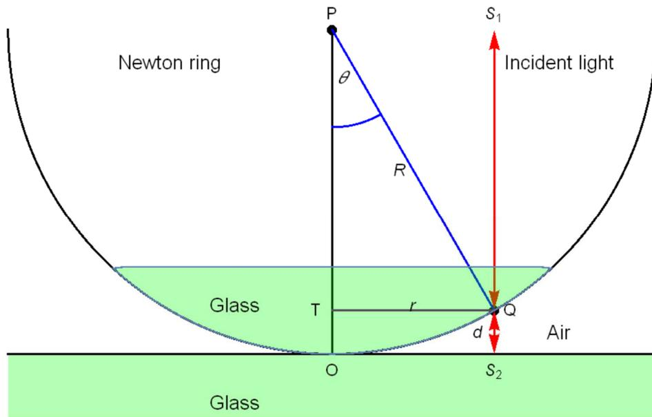
**Fig.** Newton ring. Note that the phase changes by  $\pi$  at the reflection from air to glass.
