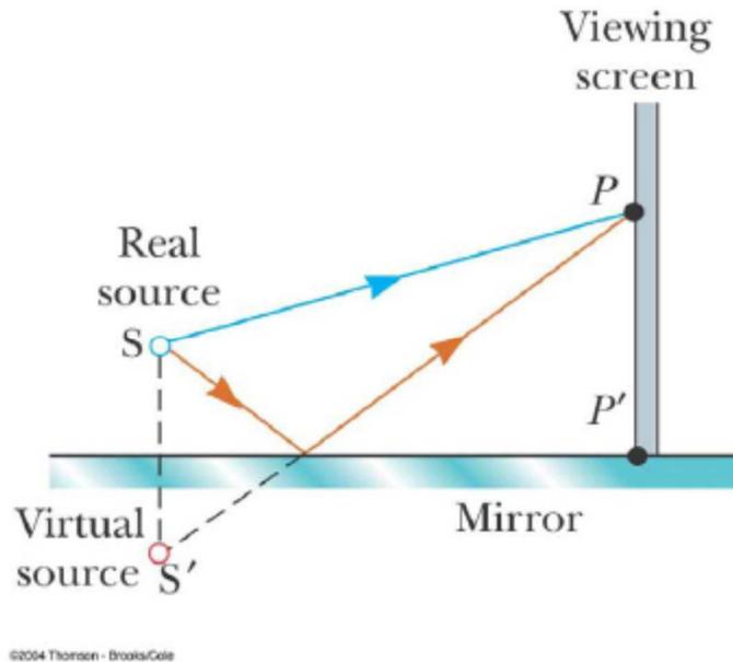
An arrangement for producing an interference pattern with a single light source. Waves reach point  $P$  either by a direct path or by reflection. The reflected ray can be treated as a ray from the source  $S'$  behind the mirror. This arrangement can be thought of as a double slit source with the distance between points  $S$  and  $S'$  comparable to length  $d$ .
