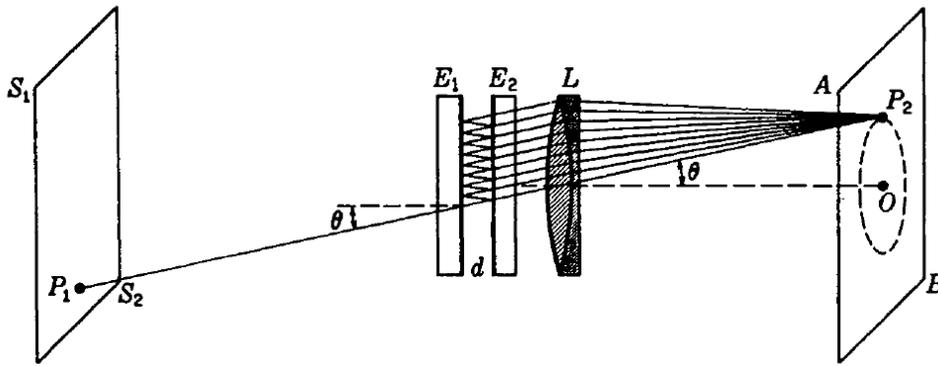
**Fig.** Fabry-Perot interferometer  $E_1E_2$  set up to show the formation of circular interference fringes from multiple reflections.
