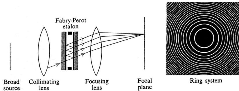
**Fig.** Arrangements for the Fabry-Perot etalon
