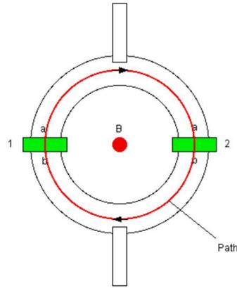
**Fig.** Schematic diagram of DC SQUID (superconducting quantum interference device).  $\delta_1$  and  $\delta_2$  refer to two point-contact weak links. The rest of the circuit is strongly superconducting.
