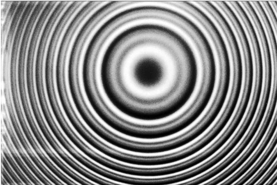
**Fig.** Interference fringes, showing fine structure, from a Fabry–Pérot etalon. The source is a cooled deuterium lamp. (Wikipedia)
