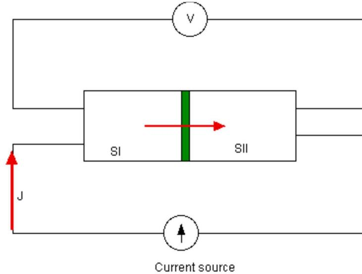
**Fig.1** Schematic diagram for experiment of DC Josephson effect. Two superconductors SI and SII (the same metals) are separated by a very thin insulating layer (denoted by green). A DC Josephson supercurrent (up to a maximum value  $I_c$ ) flows without dissipation through the insulating layer.
