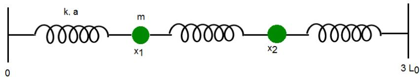
**Fig.3** A system with two masses ( $m$ ) (located at  $x = x_1$  and  $x_2$ ) and three springs with a spring constant  $k$ .  $a$  is the length of un-stretched spring. The total distance is  $3L_0$ . Both sides are fixed.
