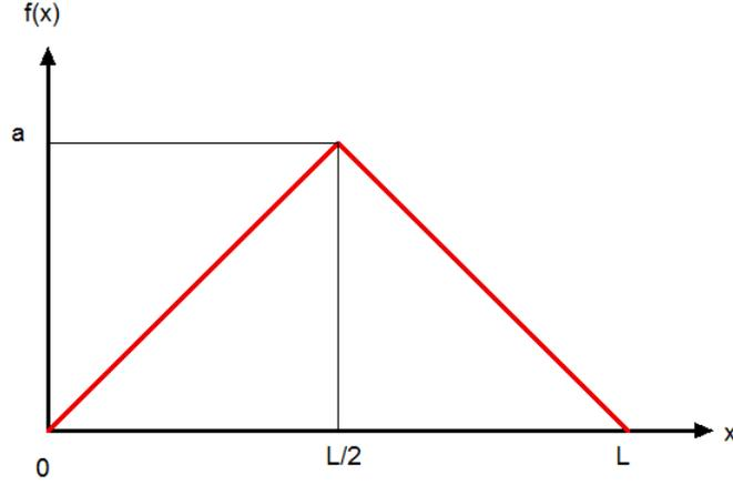
**Fig.22** Initial state of the oscillation of the string
