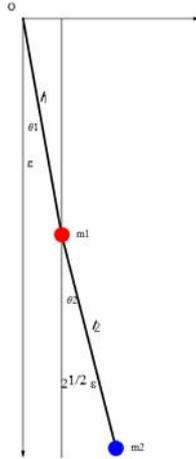
**Fig.18(a)** The initial conditions for the In-phase mode of the double pendulum. We choose the initial conditions such that  $\theta_1(t=0) = \varepsilon$ .  $\theta_2(t=0) = \sqrt{2}\varepsilon$ .  $\dot{\theta}_1(t=0) = 0$ .  $\dot{\theta}_2(t=0) = 0$ .  $\varepsilon$  is a very small angle.
