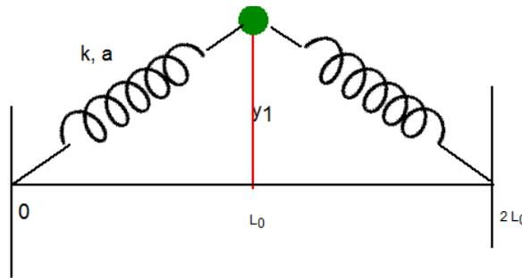
**Fig.19** Transverse oscillation for  $N = 1$  system. The displacement of the mass ( $m$ ) is restricted to the direction perpendicular to the chain in equilibrium (the length  $2L_0$ ). The spring constant is  $k$ . The length  $L_0$  is assumed to be larger than the length of un-stretched spring.
