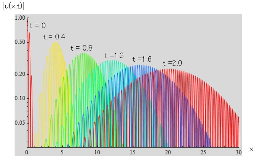
**Fig.27** Propagation pattern of the wave packet along the positive  $x$  axis at the fixed times.  $t = 0, 0.4, 0.8, 1.2, 1.6,$  and  $2.0$ .  $A_0 = 1, k_0 = 10, m = 1, \hbar = 1,$  and  $\Delta k = 3$ .
