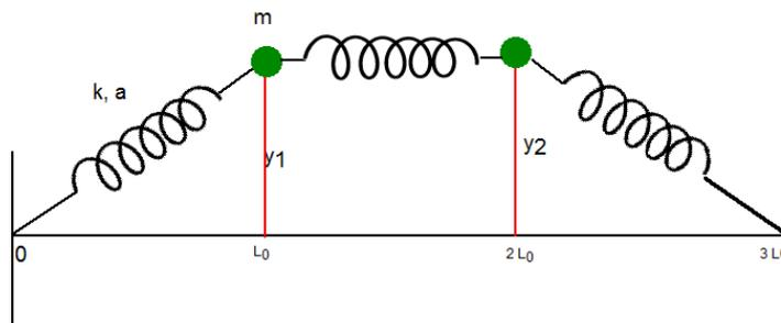
**Fig.20** Transverse oscillation for  $N = 2$  system. The displacement of each mass ( $m$ ) is restricted to the direction perpendicular to the chain in equilibrium (the length  $3L_0$ ). The spring constant is  $k$ . The length  $L_0$  is assumed to be larger than the length of un-stretched spring.
