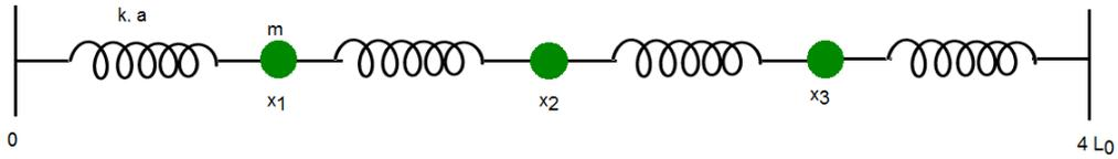
**Fig.6** A system with three masses ( $m$ ) (located at the positions  $x = x_1, x_2$ , and  $x_3$ ) and four springs with a spring constant  $k$ .  $a$  is the length of un-stretched spring. The total distance is  $4L_0$ . Both sides are fixed.
