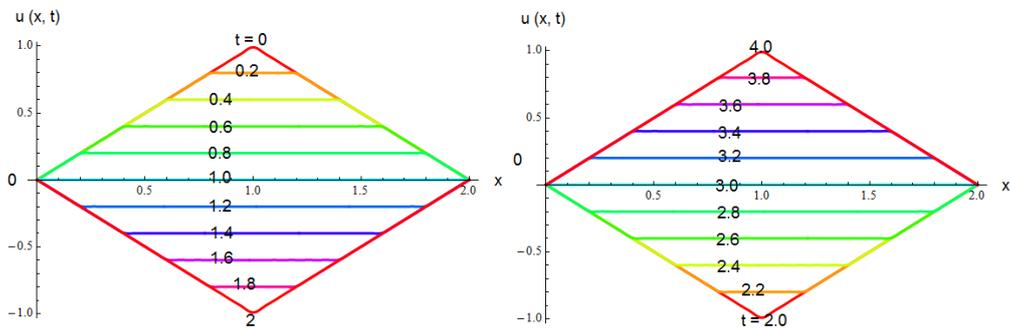
**Fig.23** Plot of  $u(x, t)$  as a function of  $x$  ( $x = 0 - 2$ ), where  $t$  is changed as a parameter ( $t = 0 - 4$ ).  $L = 2$ .  $a = 1$ .  $v = 1$ . The period  $T = 2L/v = 4$ .  $N_0 = 50$ .
