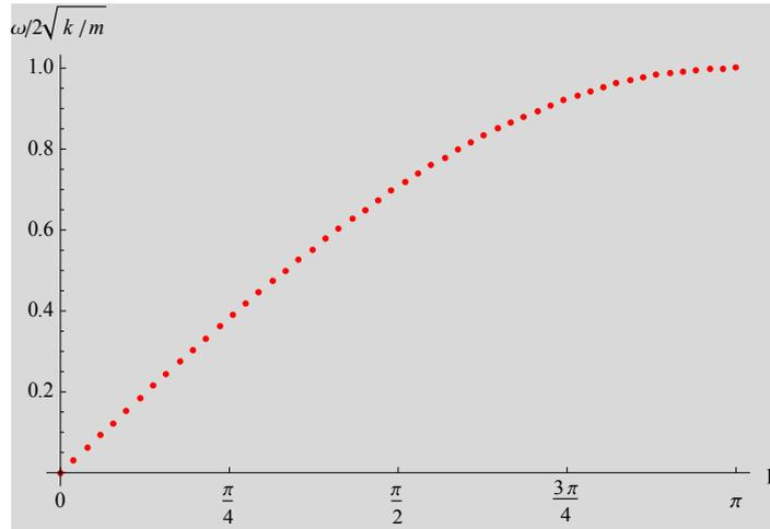
**Fig.15** Dispersion relation for  $N = 50$ . The angular frequency  $\omega_k$  vs the wave number  $p_\kappa$ .
