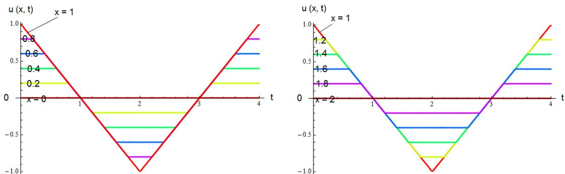
**Fig.24** Plot of  $u(x, t)$  as a function of  $t$  ( $t = 0 - 4$ ) where  $x$  is changed as a parameter ( $x = 0 - 2$ ).  $L = 2$ .  $a = 1$ .  $v = 1$ . The period  $T = 2L/v = 4$ .  $N_0 = 50$ .
