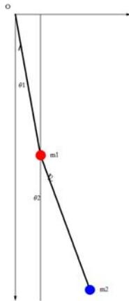
**Fig.17** Schematic diagram of the double pendulum.  $l_1 = l_2$ .  $m_1 = m_2$ .
