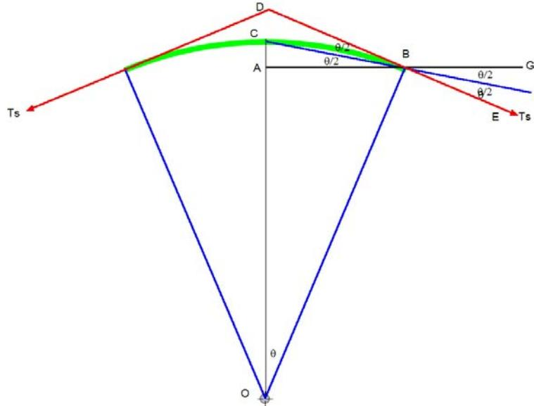
**Fig.B1** The element of string ( $\Delta s$ ) under the tension  $T = T_s$ .
