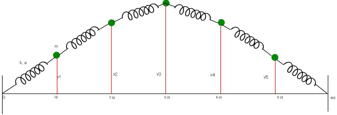
**Fig.21** Transverse oscillation for  $N = 5$  system. The displacement of each mass ( $m$ ) is restricted to the direction perpendicular to the chain in equilibrium (the length  $6L_0$ ). The spring constant is  $k$ . The length  $L_0$  is assumed to be larger than the length of un-stretched spring.
