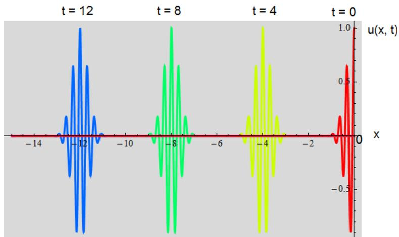
**Fig.26** Propagation of the wave packet along the negative  $x$  axis.  $A_0 = 1$ ,  $k_0 = -20$ ,  $\nu = 1$ , and  $\Delta k = 3$ .
