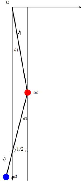
**Fig.18(b)** The initial conditions for the out-of-phase mode of the double pendulum. We choose the initial conditions such that  $\theta_1(t=0) = \varepsilon$ ,  $\theta_2(t=0) = -\sqrt{2}\varepsilon$ ,  $\dot{\theta}_1(t=0) = 0$ ,  $\dot{\theta}_2(t=0) = 0$ .  $\varepsilon$  is a very small angle.
