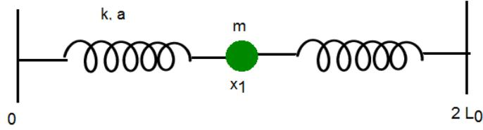
**Fig.1** A system with a mass  $m$  (located at  $x = x_1$ ) and two springs with a spring constant  $k$ .  $a$  is the length of un-stretched spring.  $x_1$  is the position of the mass along the chain. The total distance is  $2L_0$ . Both sides are fixed.
