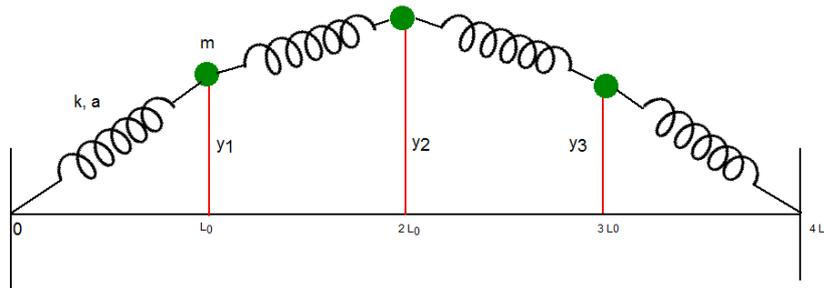
**Fig.21** Transverse oscillation for  $N = 3$  system. The displacement of each mass ( $m$ ) is restricted to the direction perpendicular to the chain in equilibrium (the length  $4L_0$ ). The spring constant is  $k$ . The length  $L_0$  is assumed to be larger than the length of un-stretched spring.
