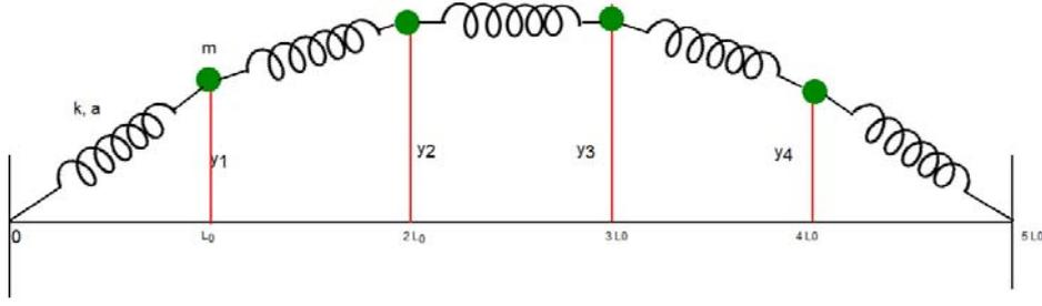
**Fig.22** Transverse oscillation for  $N = 4$  system. The displacement of each mass ( $m$ ) is restricted to the direction perpendicular to the chain in equilibrium (the length  $5L_0$ ). The spring constant is  $k$ . The length  $L_0$  is assumed to be larger than the length of un-stretched spring.
