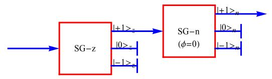
Two Stern-Gerlach type filters in series; the second is tilted at the angle  $\theta$  from the z axis in the x-z plane.
