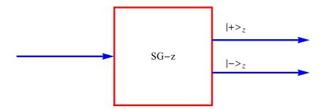
The beam is then expected to get slit according to the values of  $\mu$  (or  $S_z$ ). In other words, the SG apparatus measures the z-component of  $\mu$ , or equivalently, the z-component of S.
