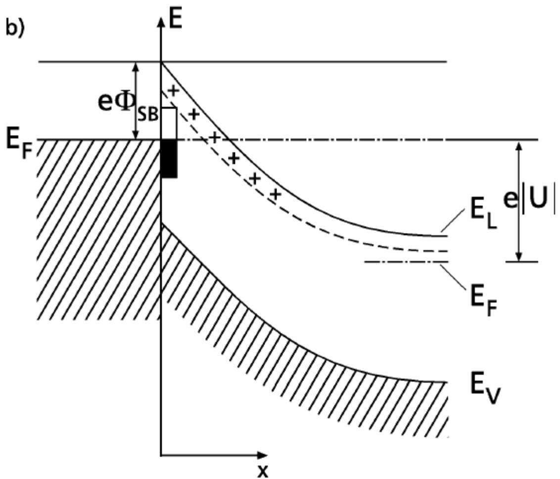
**Fig. 12.22.** Electronic band scheme of a metal/semiconductor (*n*-doped) junction; pinning of the Fermi-level  $E_F$  in interface states near the neutrality level causes the formation of a Schottky-barrier  $e\phi_{SB}$  and a depletion space charge layer within the semiconductor.  $V_D$  is the “built-in” diffusion voltage. **(a)** In thermal equilibrium, **(b)** under external bias  $U$
