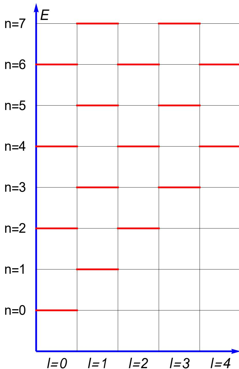
**Fig.** The energy levels  $E_n = (n + \frac{3}{2})\hbar\omega$  of the 3D isotropic simple harmonics, showing the degeneracy. The degeneracy is 1 ( $n = 0$ ), 3 ( $n = 1$ ), 6 ( $=1 + 5$ ) ( $n = 2$ ), 10 ( $=3 + 7$ ) ( $n = 3$ ), 15 ( $=1 + 5 + 9$ ) ( $n = 4$ ), 21 ( $n = 5$ ), 28 ( $n = 6$ ).
