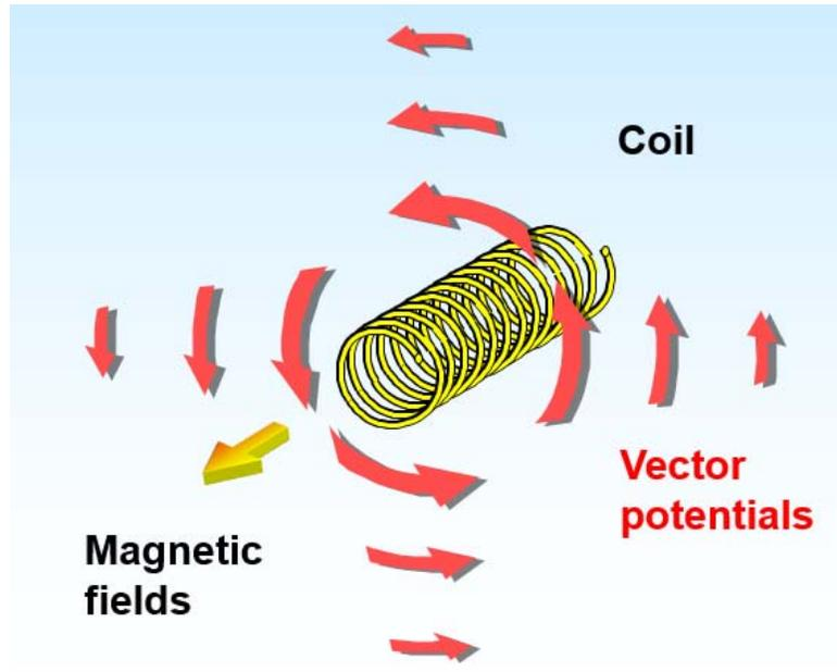
**Fig.** The direction of the vector potential around the solenoid coil.
