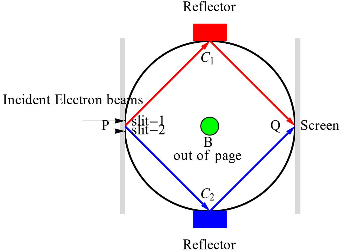
**Fig.** Schematic diagram of the Aharonov-Bohm experiment. Incident electron beams go into the two narrow slits (one beam denoted by blue arrow, and the other beam denoted by red arrow). The diffraction pattern is observed on the screen. The reflector plays a role of mirror for the optical experiment.
