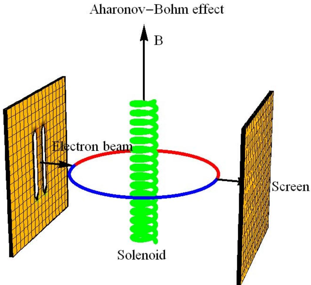
**Fig.** Schematic diagram of the Aharonov-Bohm experiment. Electron beams are split into two paths that go to either a collection of lines of magnetic flux (achieved by means of a long solenoid). The beams are brought together at a screen, and the
