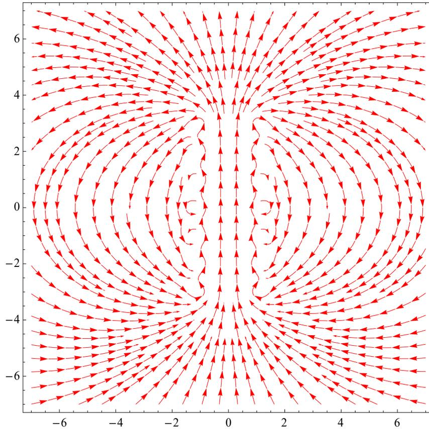
**Fig.** Magnetic field lines of the system of 7 current loops stacked along the  $z$  axis, which are equally spaced. When the coil is wound tightly and there are more loops, the magnetic field inside become larger and more uniform. The magnetic field  $\mathbf{B}$  forms a closed loop.
