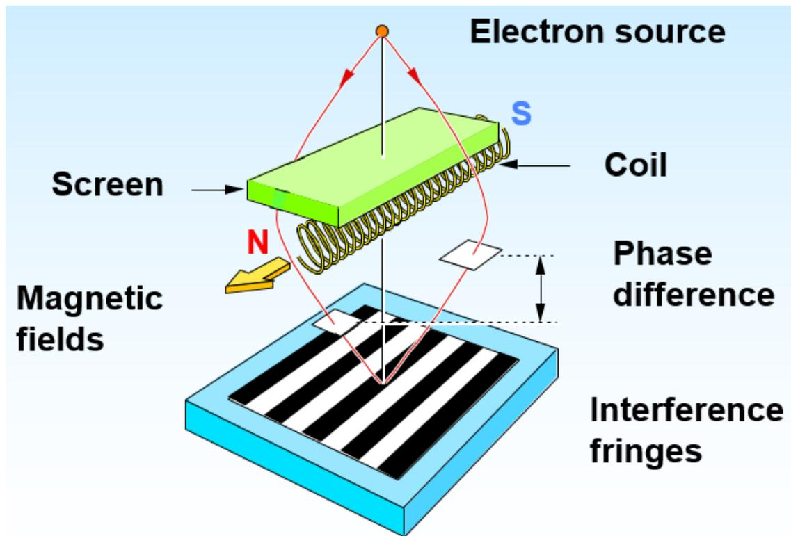
**Fig.** Schematic diagram of the Aharonov-Bohm effect (by A. Tonomura group at Hitachi).
