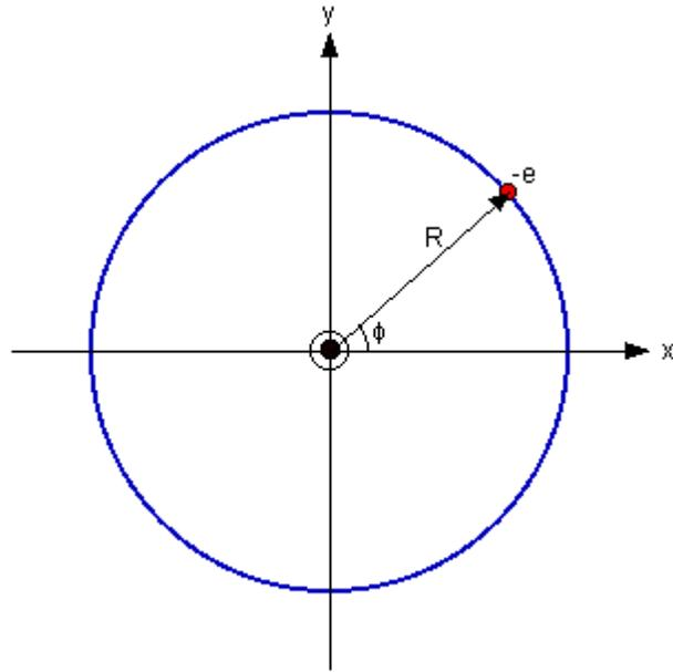
**Fig.** Circular conducting ring with radius  $R = \rho$ . The magnetic field  $\mathbf{B}$  is located only at the center and is along the  $z$  axis (out of the page).
