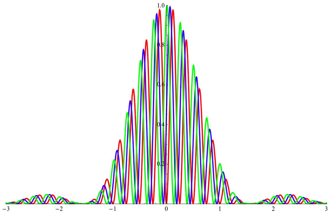
Fig. Young's double slits diffraction with Aharonov-Bohm effect. The diffraction pattern changes with the magnetic field. red ( $B = 0$ ). Blue ( $B$ =intermediate value). Green ( $B$  = stronger field).
