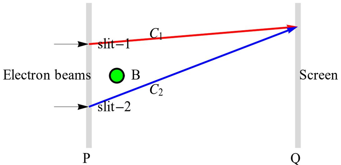
**Fig.** Young's double slit experiment with the electron beam source. The magnetic field is applied just behind the slits. There is no magnetic field around the paths ( $C_1$  and  $C_2$ ).
