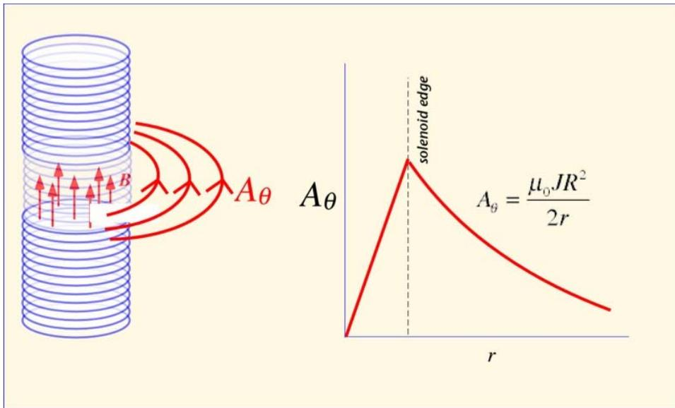
**Fig.** The vector potential distribution around the solenoid.
