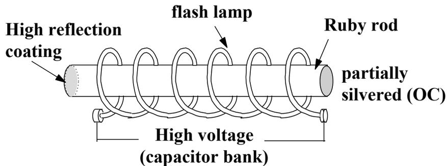
**Fig.** The first laser invented (in 1960). Pump source: flash lamp. Classic 3-level laser. Very low repetition rate  $\sim 1$  pulse/min. Since its repetition rate is so slow, nobody wants to use this type of laser these days. Laser wavelength 694.3 nm, pulse width  $\sim 10^{-8}$  sec.
