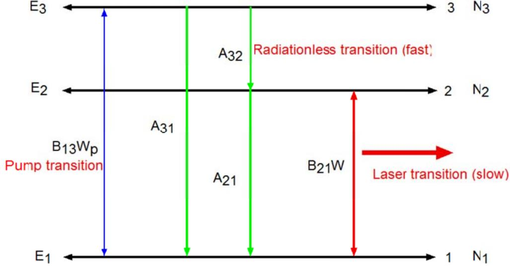
**Fig.** A transition in the three-level laser. The lasing transition takes the system from the metastable state ( $E_2$ ) to the ground state ( $E_1$ ). The population inversion occurs when  $A_{32} \gg A_{21}$  (or  $\tau_{21} \gg \tau_{32}$ )
