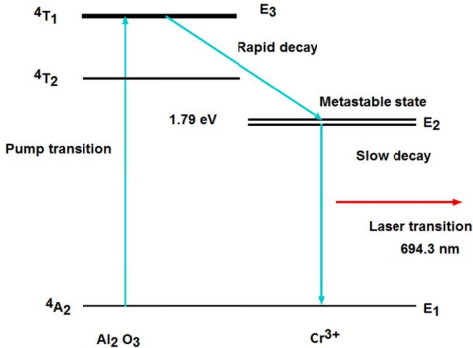
**Fig.** Laser transition for Ruby laser.  $\lambda = 694.3\text{ nm}$ .
