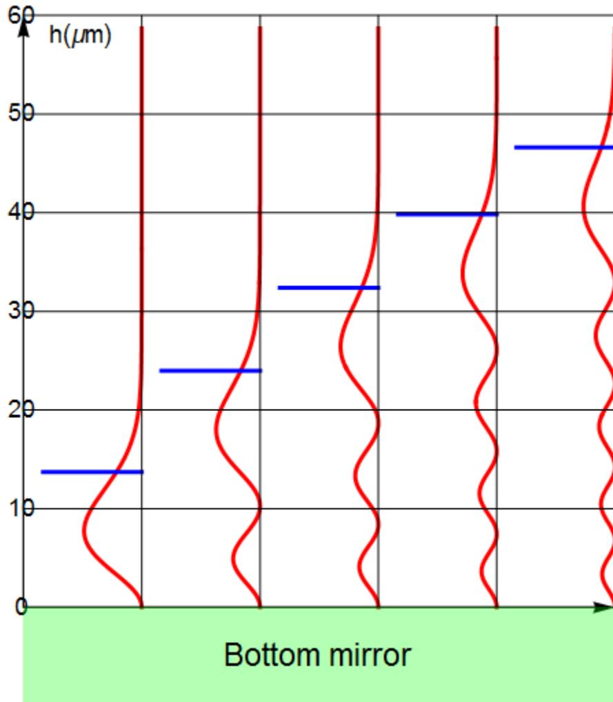
**Fig.** Probability amplitude  $\psi_n^2(x)$  for the  $n$ -th state ( $n = 1, 2, 3, \dots$ ). The blue lines denote the turning point in the classical limit. The energy eigenvalue of the  $n$ -th state is given by  $mga_n$  where  $a_n$  is the height of the turning point. The wave function has an odd parity since it should be zero at  $x = 0$  because of the infinite potential at  $x = 0$ .
