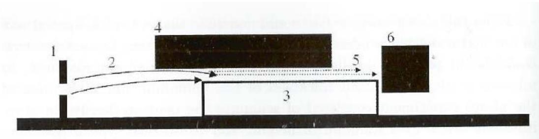
**Fig:** A simplified scheme of measuring gravitational quantum states of neutrons.
