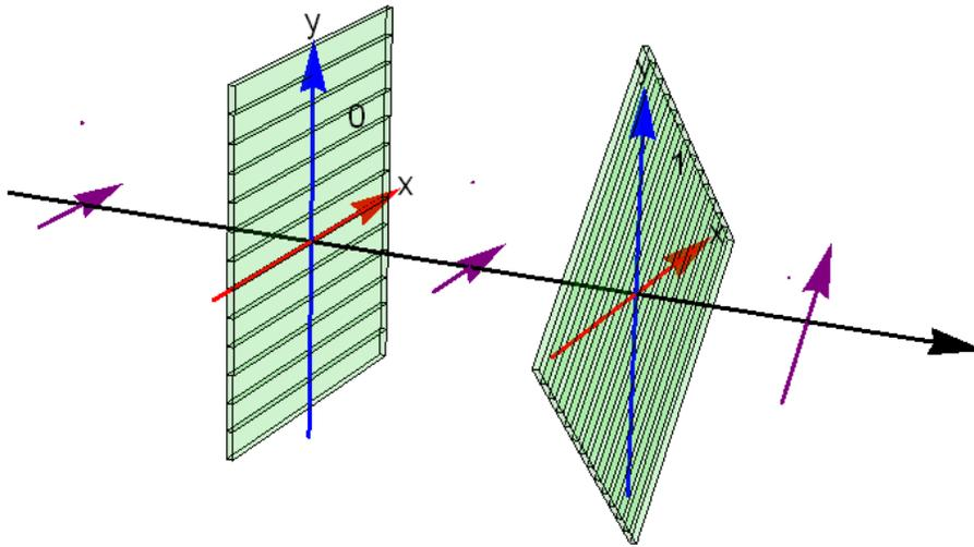
**Fig.** The light with the polarization  $|x\rangle$  passes through a filter with  $|\theta\rangle$ .
