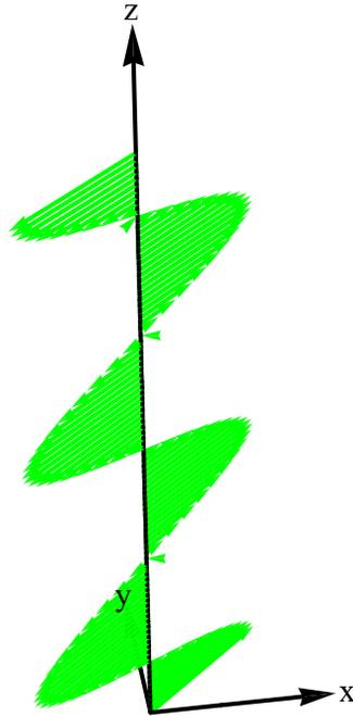
**Fig.** Linear polarization (45° polarization). ParametricPlot3D of  $\{\cos(kz), \cos(kz), z\}$ , where  $z$  is varied as a parameter between  $z = 0$  and  $z = 5.k = \pi$ . In this case,  $t = 0$ .
