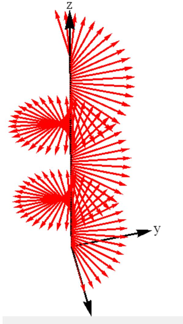
**Fig.** Left circularly polarization with  $z$ . ParametricPlot3D of  $\left\{ \frac{1}{\sqrt{2}} \cos(kz), \frac{1}{\sqrt{2}} \sin(kz), z \right\}$ , where  $z$  is varied as a parameter between  $z = 0$  and  $z = 5$ .  $k = \pi$ . Note that  $t$  is fixed. In this case  $t = 0$ . The electric field rotates in a **counterclock-wise direction** as  $z$  is increased.
