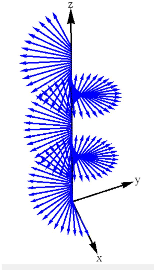
**Fig.** Right circularly polarization with  $z$ . ParametricPlot3D of  $\left\{ \frac{1}{\sqrt{2}} \cos(kz), -\frac{1}{\sqrt{2}} \sin(kz), z \right\}$ , where  $z$  is varied as a parameter between  $z = 0$  and  $z = 5.k = \pi$ . Note that  $t$  is fixed. In this case,  $t = 0$ . The electric field rotates in a **clock-wise direction** as  $z$  is increased.
