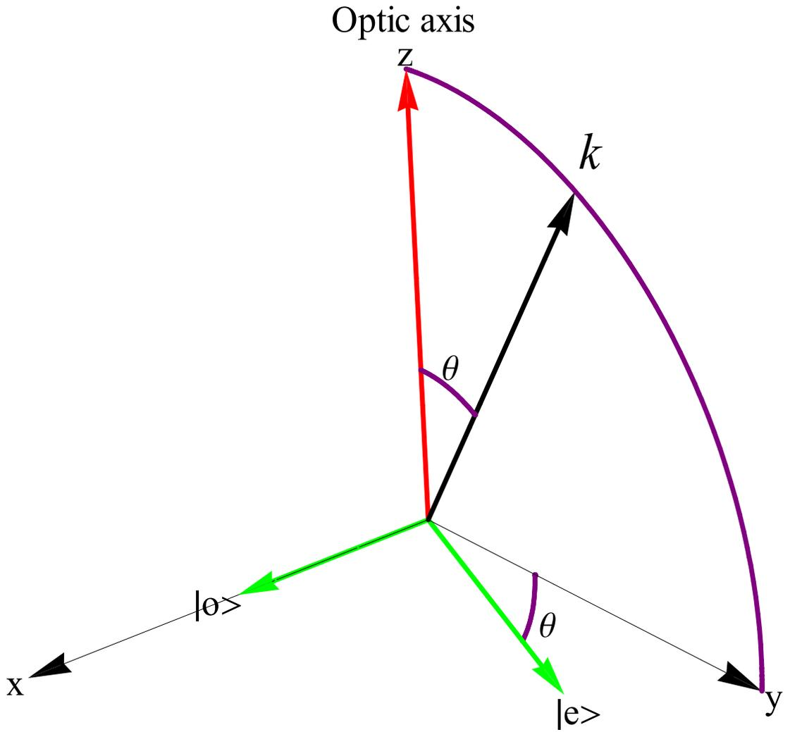
**Fig.** Electric field vector of ray propagating in a uniaxial crystal with its optic axis along the  $z$  axis. The ray with the wavevector  $k$  makes an angle of  $\theta$  with respect to the optic axis (the  $z$ -axis). The  $x$  and  $y$  axes are chosen so that the beam is propagating in the  $y$ - $z$  plane.
