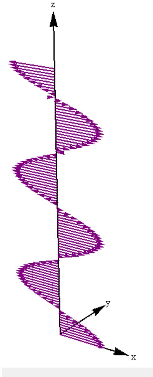
**Fig.** Linear polarization with  $z$ . ParametricPlot3D of  $\{\cos(kz), 0, z\}$ , where  $z$  is varied as a parameter between  $z = 0$  and  $z = 5.k = \pi$ . Note that  $t$  is fixed. In this case,  $t = 0$ .
