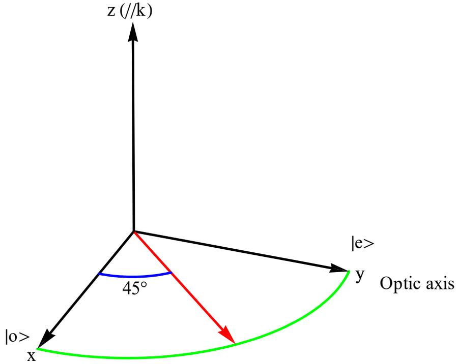
The index refraction is  $n_y$  for the  $e$ -ray and  $n_x$  for the  $o$ -ray;  $n_y > n_x$ . The crystal can be cut to a particular thickness  $z$ , called a quarter-wave plate.
