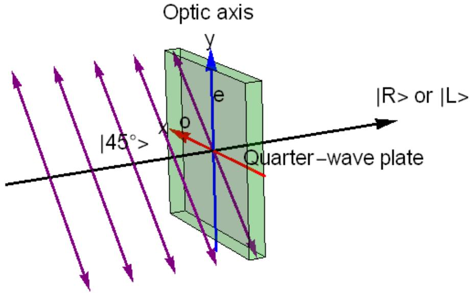
**Fig.** If linearly polarized light is incident on a quarter-wave plate at  $45^\circ$  to the optic axis, then the light is divided into two equal electric field components. One of these is retarded by a quarter wavelength by the plate. This produces circularly polarized light. Incident circularly polarized light will be changed to linearly polarized light.
