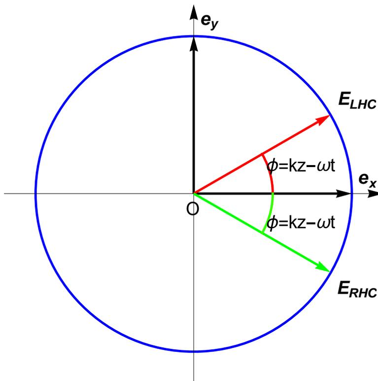
**Fig.** Direction of the electric field for the RHC (right-hand circularly) photon and LHC (left-hand circularly) photon ( $x$ - $y$  plane which is perpendicular to the propagation direction  $z$  axis). The phase angle is given by  $\phi = kz - \omega t$ .
