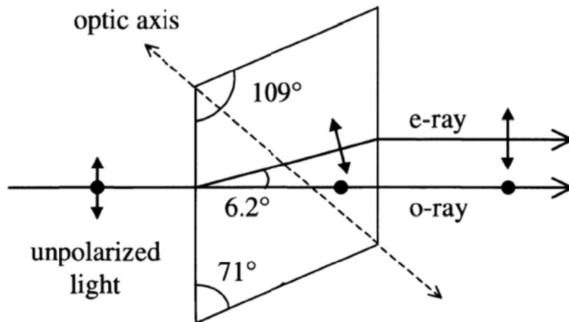
**Fig.** A light with two orthogonal field components traversing a calcite section. (M. Fox, *Optical Properties of Solids* (Oxford, 2001).
