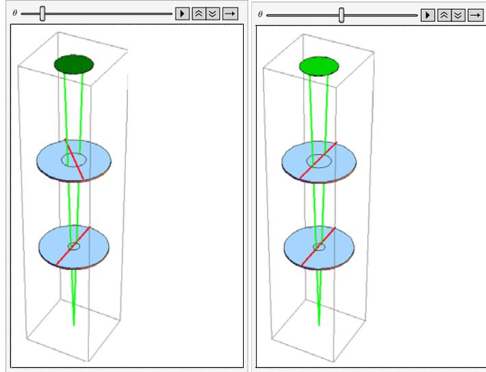
**Fig.** Demonstration for the role of two polarizers. The light passes when the directions of the two polarizers are the same. The light does not pass when the directions of two polarizers are perpendicular to each other.
