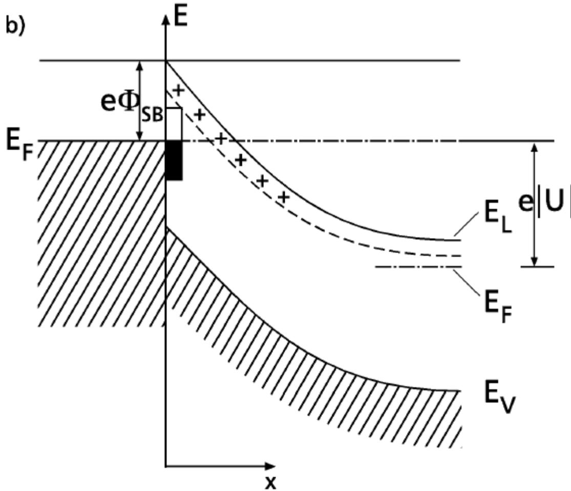
**Fig.** Electronic band scheme of a metal/semiconductor (n-doped) junction: pinning of the Fermi-level  $E_F$  in interface states near the neutrality level causes the formation of a Schottky-barrier  $e\phi_{SB}$  and a depletion space charge layer within the semiconductor.  $V_D$  is the built-in diffusion voltage. (a) In thermal equilibrium, (b) under external bias  $U$ .
