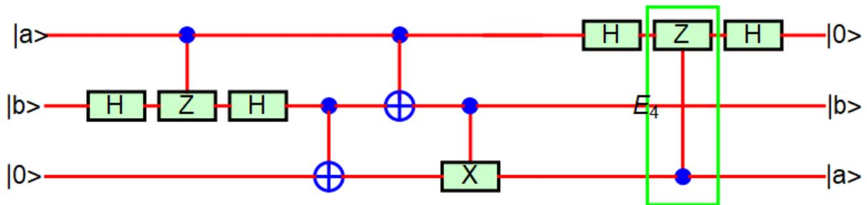
**Fig.31 (c):** Controlled Z is nonlocal in the elements  $E_4$ . Even if the location of the control and target is changed, the role of CZ remains unchanged.
