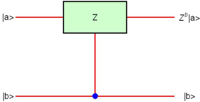
**Fig.15(b)** Controlled Z gate. Control gate ( $|b\rangle$ ) and target gate ( $|a\rangle$ ).  $Z^b |a\rangle \otimes |b\rangle = (-1)^{ab} |a\rangle \otimes |b\rangle$ . Figs.15(a) and 15(b) are equivalent. CZ gate is non-local, independent of the choice of control and target.
