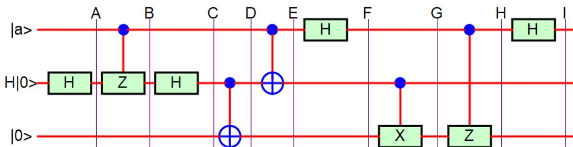
**Fig.32** The equivalent quantum circuit for the SWAP.
