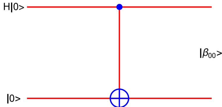
**Fig.6** Encode of the Bell state  $|\beta_{00}\rangle$  using CNOT gate with control ( $H|0\rangle$ ) and target ( $|0\rangle$ ).
