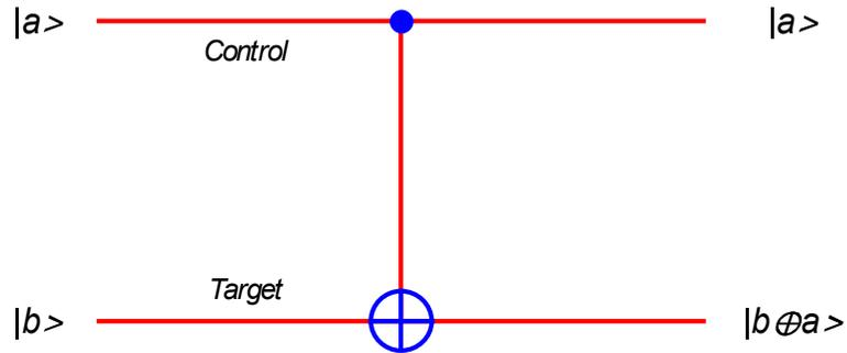
**Fig.4** Controlled Not gate (CNOT).  $|a\rangle$ : control.  $|b\rangle$ : target.
