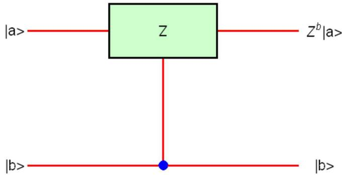
**Fig.8(b)** Controlled Z gate with control ( $|b\rangle$ ) and target ( $|a\rangle$ ), which is equivalent to Fig.8(a)
