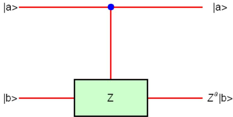
**Fig.27** Controlled Z gate.  $Z^a |b\rangle = (-1)^{ab} |b\rangle$ .
