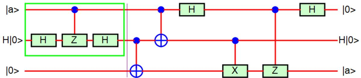
**Fig.35** No change occurs to the circuit upon the removal of the circuit element enclosed by the green box.
