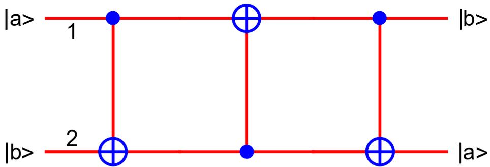
**Fig.7(b)** Circuit equivalent to SWAP circuit.
