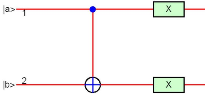
**Fig.13(b)** Quantum circuit equivalent to Fig.13(a).
