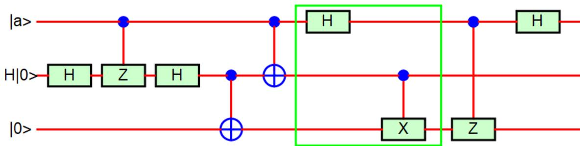
**Fig.31(f):** The circuit after shifting H and CX within the green box. The input:  $|a\rangle$  for Charlie. The input:  $|0\rangle$  for Bob. For simplicity, we choose the input  $H|0\rangle$  for Alice. This input is arbitrary.  $H|0\rangle_A = \frac{1}{\sqrt{2}}[|0\rangle_A + |1\rangle_A]$ .
