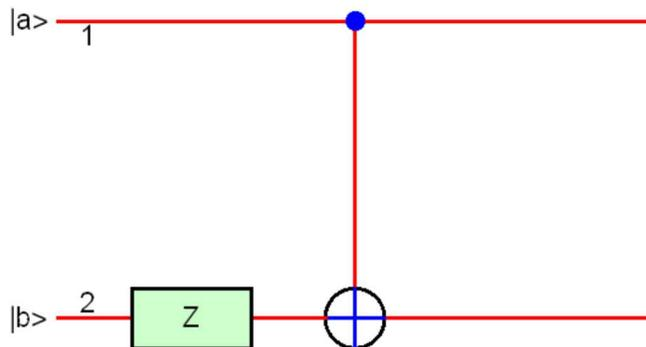
**Fig.12(a)** Quantum circuit-2
