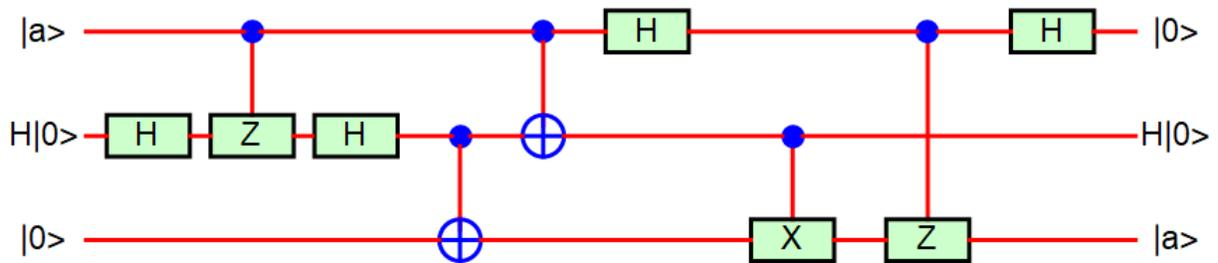
**Fig.34** SWAP. The output:  $|0\rangle_C$ ,  $H|0\rangle_A$ , and  $|a\rangle_B$ . The input:  $|a\rangle_C$ ,  $H|0\rangle_A$ , and  $|0\rangle_B$ .
