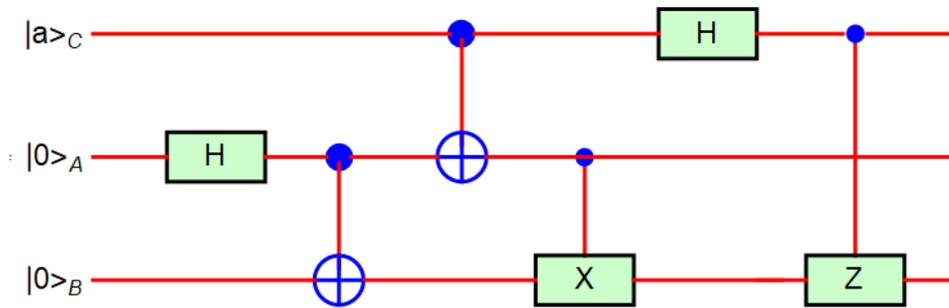
**Fig.21** The circuit as input with the states  $|a\rangle$  (Charlie),  $|0\rangle$  (Alice), and  $|0\rangle$  (Bob).
