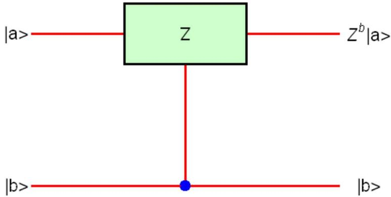
**Fig.28**  $Z^b |a\rangle = (-1)^{ab} |a\rangle$ . CZ (controlled Z) is nonlocal, independent of the choice of the control and the target.
