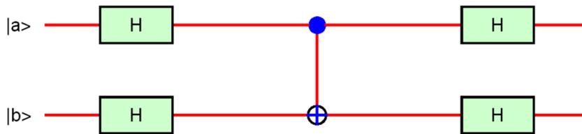
**Fig.16(a)** Quantum circuit-6, with 4  $H$ -gates and 1  $CZ$ -gate. Control gate ( $|a\rangle$ ) and target gate ( $|b\rangle$ ). Input:  $|a\rangle \otimes |b\rangle$ . Output:  $|a \oplus b\rangle \otimes |b\rangle$ .
