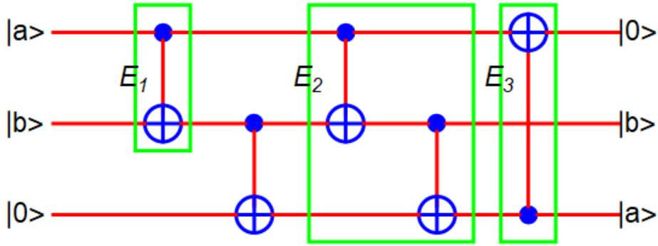
**Fig.26** In SWAP, the circuit elements  $E_1$ ,  $E_2$ , and  $E_3$  can be replaced by the corresponding equivalent circuits.
