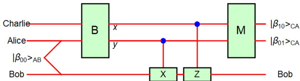
**Fig.18** Quantum teleportation circuit (Alice, Bob, and Charlie). The box B denotes the generation of the Bell state. The box M denotes the measurement
