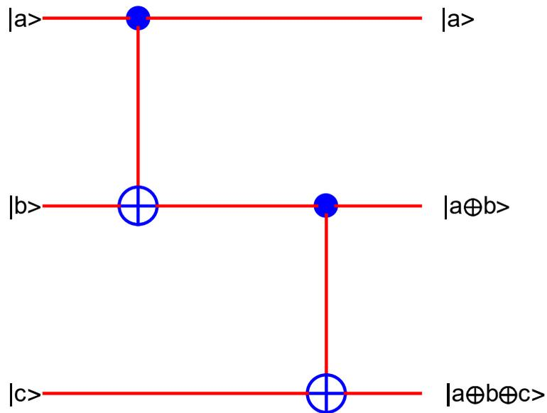
**Fig.29** The circuit of Fig.31 is equivalent to that in Fig.32.
