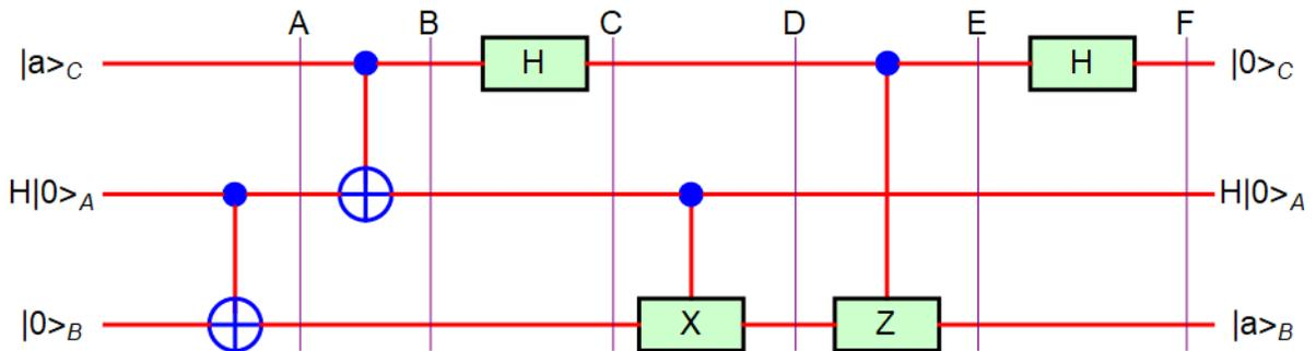
**Fig.37** The output after the step  $E$ ;  $\frac{1}{\sqrt{2}}[|\beta_{00}\rangle_{CA} + |\beta_{01}\rangle_{CA}] \otimes |a\rangle$ . Immediately after Alice measures one of the Bell states ( $|\beta_{00}\rangle_{CA}, |\beta_{01}\rangle_{CA}$ ), the state of Bob collapse into the state  $|a\rangle$ . The output after the step  $F$ ;  $|0\rangle_C \otimes H|0\rangle_A \otimes |a\rangle_B$ .
