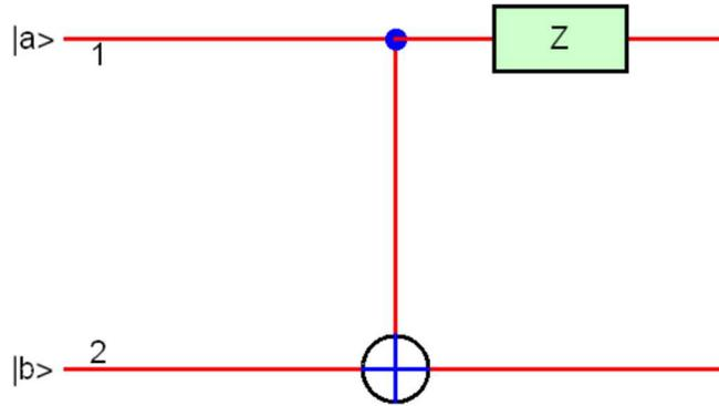
**Fig.14(b)** CNOT and Z-gate. Quantum circuit equivalent to the quantum circuit -4 of Fig.14(a). 1: control. 2: target. Input:  $|a\rangle \otimes |b\rangle$ . Output:  $(-1)^a |a\rangle \otimes |a \oplus b\rangle$ . Figs.14(a) and (b) are equivalent.
