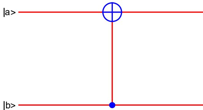
**Fig.16(b)** *CNOT* gate. Quantum circuit equivalent to Fig.16(a). Control gate ( $|b\rangle$ ) and target gate ( $|a\rangle$ ). The input: Input:  $|a\rangle \otimes |b\rangle$ . Output:  $|a \oplus b\rangle \otimes |b\rangle$ .
