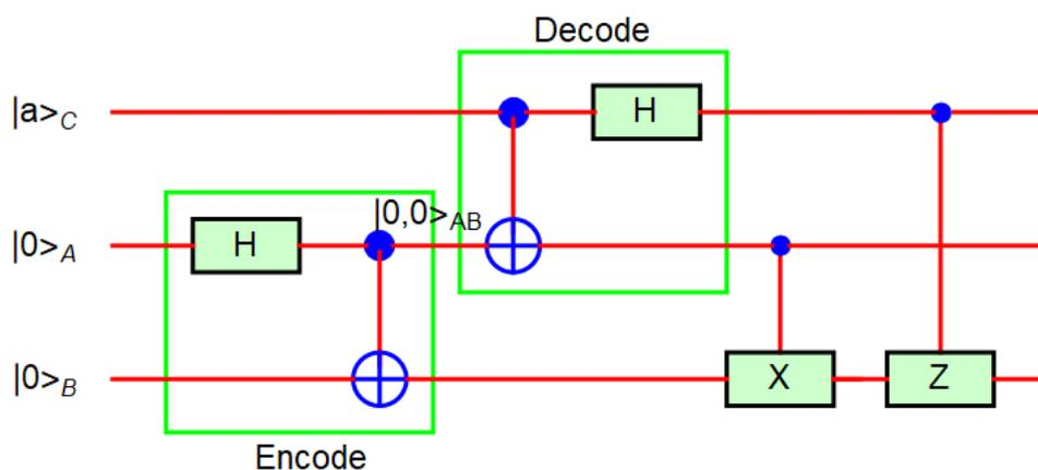
**Fig.19** Equivalent quantum circuit of quantum teleportation, with encode of Bell state  $|\beta_{00}\rangle$  and decode of the Bell state.
