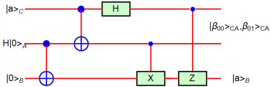
**Fig.38** Equivalent circuit both for the quantum teleportation and the SWAP.
