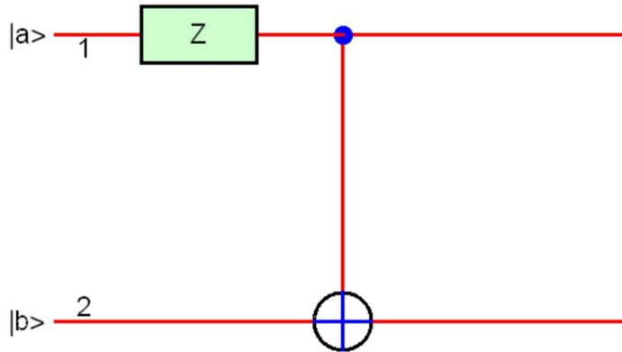
**Fig.14(a)** Z-gate and CNOT. Quantum circuit-4. 1: control. 2: target. Input:  $|a\rangle \otimes |b\rangle$ .
