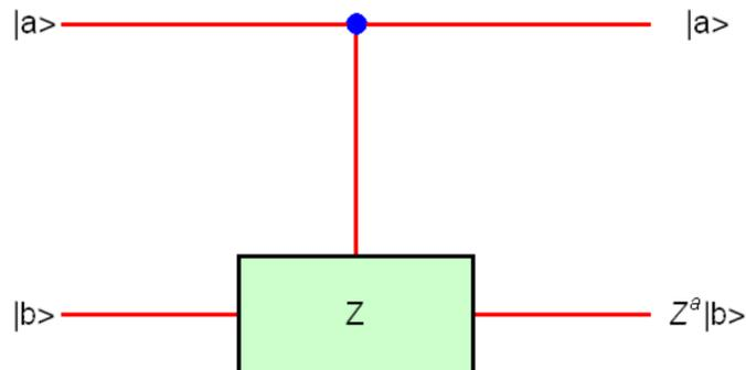
**Fig.15(a)** Controlled Z gate. Quantum circuit-5. Control gate ( $|a\rangle$ ) and target gate ( $|b\rangle$ ). 1: control ( $|a\rangle$ ). 2: target ( $|b\rangle$ ). Input:  $|a\rangle \otimes |b\rangle$ . Output:  $(-1)^{ab} |a\rangle \otimes |b\rangle$ .
