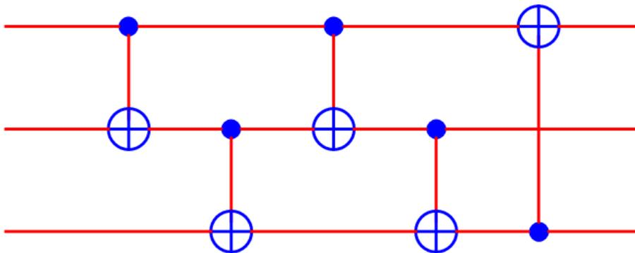
**Fig.24(b)** Equivalent circuit of SWAP, where the SWAP is replaced by CNOTs.
