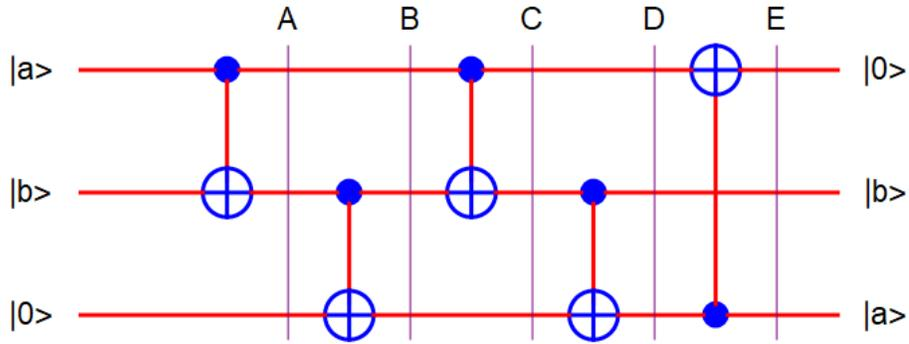
**Fig.25** The same circuit as Fig.26(b), with input ( $|a\rangle$  for Charlie, for Alice  $|b\rangle$ , and  $|0\rangle$  for Bob).
