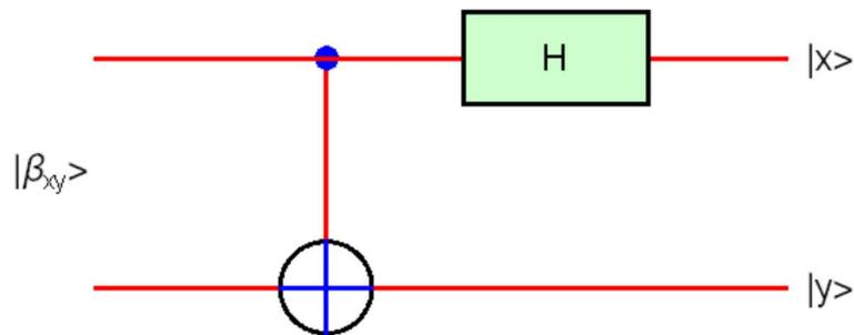
**Fig.10** Decode of Bell state  $|\beta_{xy}\rangle$ . Base transformation  $(|x\rangle \otimes |y\rangle) \rightarrow |\beta_{xy}\rangle$  by H-CNOT gate.
