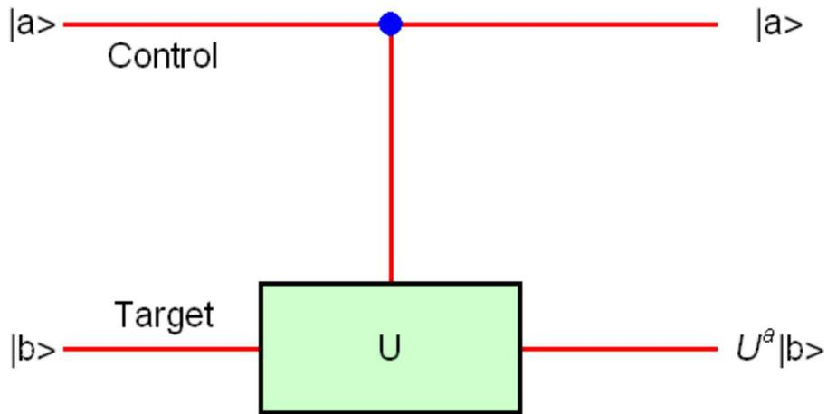
**Fig.2** Controlled  $U$  gate. Control ( $|a\rangle$ ). Target ( $|b\rangle$ ).
