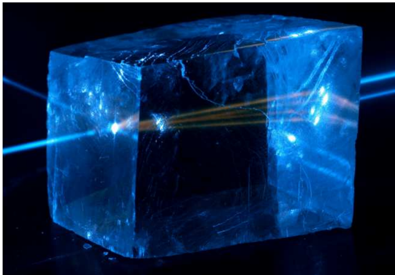
Fig.5 Birefringence in calcite crystal as laser beam splits into two rays ( o -wave and e -wave) while travelling from left to light. (Wikipedia).
