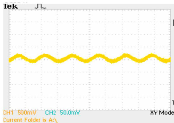
Fig. 8 The V - \Phi curve to determine the modulation depth
