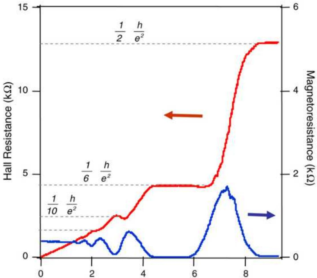
Fig. Quantized magnetoresistance and Hall resistance of a graphene device where  $n = 10^{12} \text{ cm}^{-2}$  and  $T = 1.6 \text{ K}$ . Z. Jiang et al. Solid State Commun. 143, 14-19 (2007).
