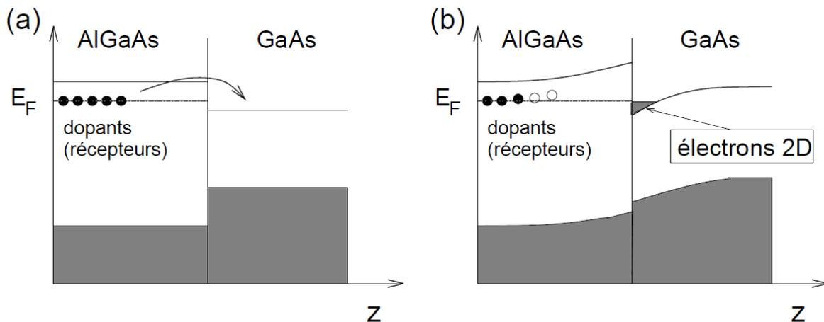
**Fig.** Semiconducting (GaAs/AlGaAs) heterostructure. (a) A layer of (receptor) dopants lies on the AlGaAs side, at a certain distance from the interface. The Fermi energy is locked to the dopant levels. The bottom of the GaAs conduction band lies lower
