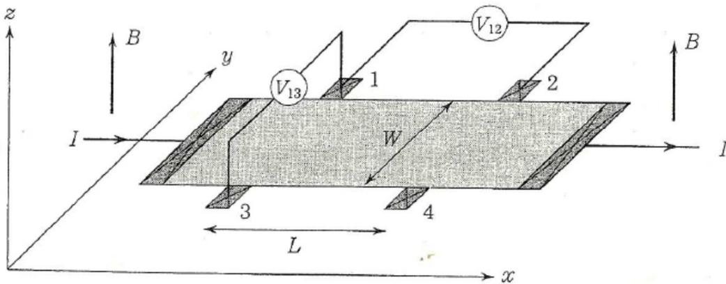
Fig. Measurement of the Hall and diagonal resistivities.
