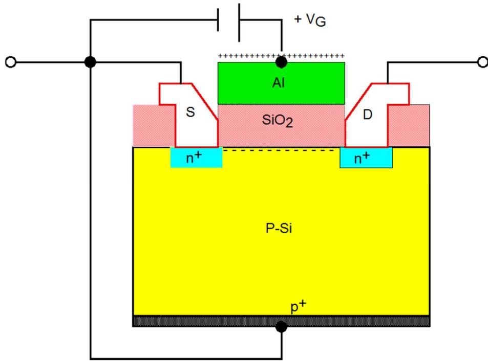
The source S and drain D contacts are heavily doped n<sup>+</sup> regions with Al caps.
