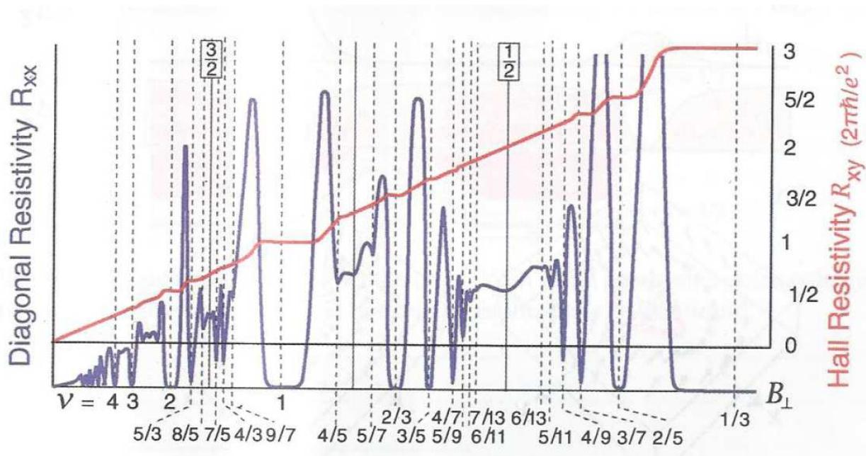
Fig. Quantum Hall effect which are detected by plateau developed by the Hall resistivity or dips in the diagonal resistivity. The numbers indicate the Landau level filling factors at which various features occur,
