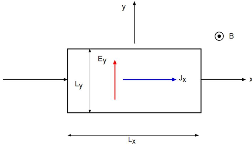
**Fig.** Experimental configuration for the measurement of Hall effect.
