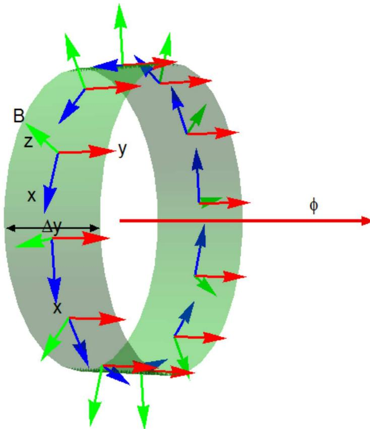
When  $\Delta y = \frac{2\Phi_0}{LB}$ , the total magnetic flux passing through the cylinder surface (along the  $z$  axis, the direction of the magnetic field  $\mathbf{B}$ ) is  $2\Phi_0$ . Note that total surface area of the cylinder is
