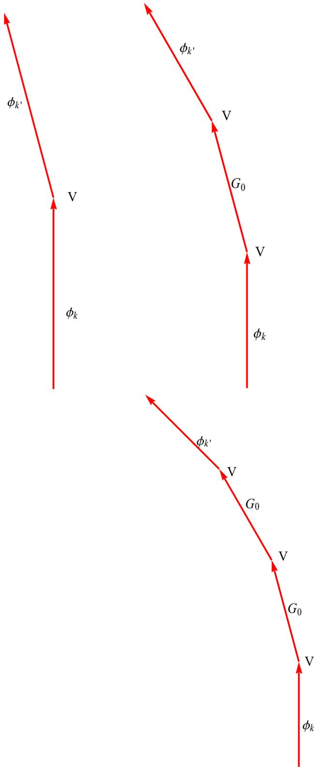
**Fig.** Feynman diagram. First order, 2nd order, and 3rd order Born approximations.  $\phi_k = |\mathbf{k}\rangle$  is the initial state of the incoming particle and  $\phi_{k'} = |\mathbf{k}'\rangle$  is the final state of the incoming particle.  $\hat{V}$  is the interaction.
