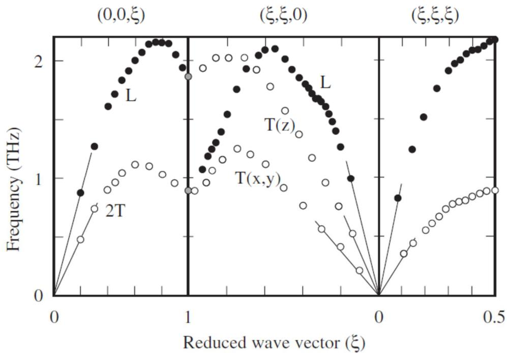
**Fig.** Acoustic mode dispersion curves for lead (fcc) measured by inelastic scattering (Data taken from Brockhouse et al. Phys. Rev. **128**, 1099, 1962). M.T. Dove, Structure and Dynamics: An Atomic View of Materials (Oxford, 2002).
