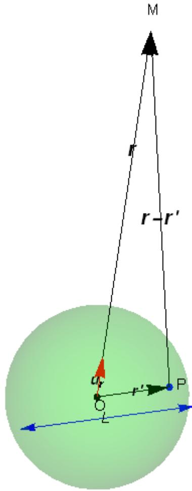
**Fig.** Vectors  $r$  and  $r'$  in calculation of scattering amplitude in the first Born approximation
