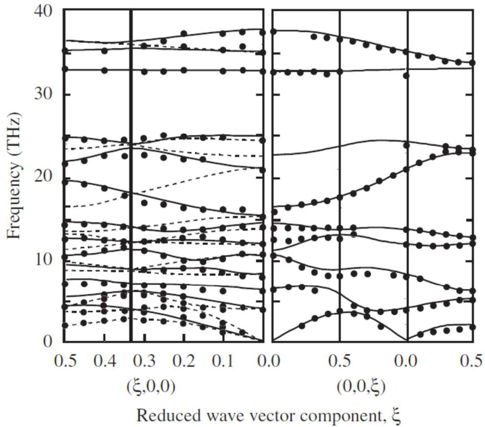
**Fig.** Dispersion curves for quartz. (Data are taken from Strauch and Dorner, *J. Phys. Cond. Matter* **5**, 6149, 1993). M.T. Dove, *Structure and Dynamics: An Atomic View of Materials* (Oxford, 2002).
