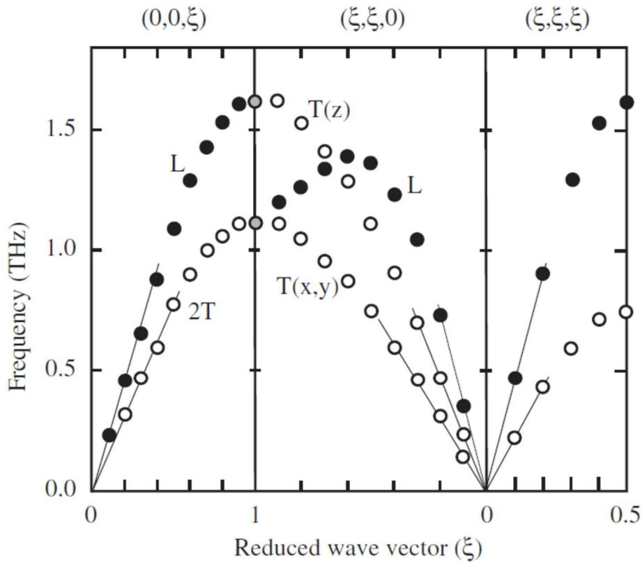
**Fig.** Acoustic mode dispersion curves for neon (ccp structure) measured by inelastic neutron scattering. (Data taken from Endoh et al. Phys. Rev. B11, 1681, 1975). M.T. Dove, Structure and Dynamics: An Atomic View of Materials (Oxford, 2002).
