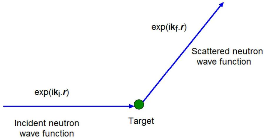
**Fig.** Schematic diagram for the neutron scattering,  $\mathbf{Q} = \mathbf{k}_i - \mathbf{k}_f$ .  $k_i = k$ .  $k_f = k'$ .
