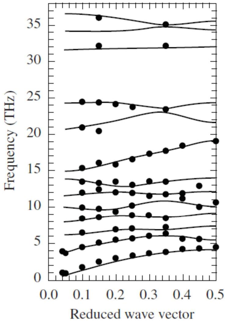
**Fig.** Phonon dispersion curves of quartz obtained by inelastic x-ray scattering. (Data from Ch. Halcoussis, *J. Phys.,: Cond. Matter* 13, 7627, 2001).
