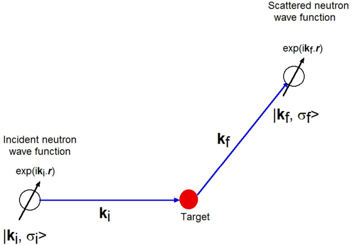
Fig. Scattering of neutron by a target.  $k_i = k'$ .  $k_f = k'$ . The scattering vector  $Q = k_i - k_f$ .
