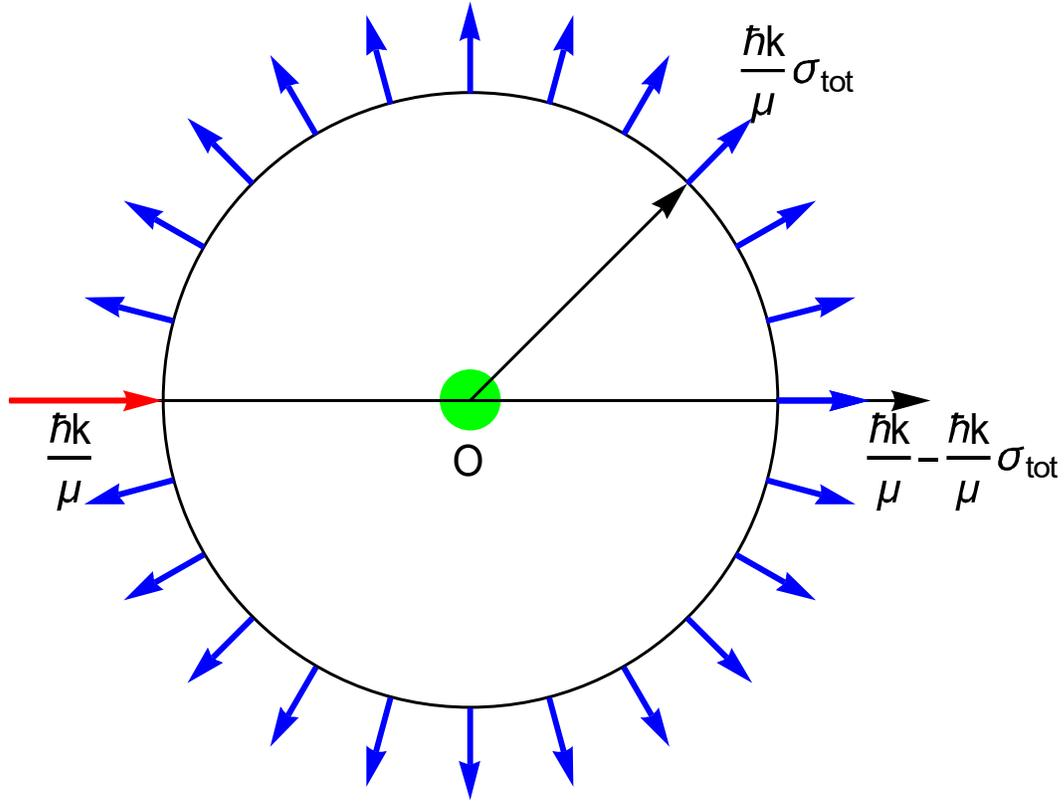
**Fig.** Optical theorem. The intensity of the incident wave is  $\hbar k / \mu$ . The intensity of the forward wave is  $(\hbar k / \mu) - (4\pi\hbar / \mu) \text{Im}[f(0)]$ . The waves with the total intensity  $(4\pi\hbar / \mu) \text{Im}[f(0)] = (\hbar k / \mu)\sigma_{tot}$  is scattered for all the directions, as the scattering spherical waves.
