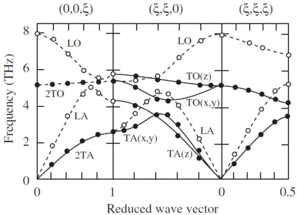
**Fig.** Dispersion curves for NaCl (inelastic neutron scattering). (Data taken from Raunio et al. Phys. Rev. **178**, 1496, 1969). M.T. Dove, Structure and Dynamics: An Atomic View of Materials (Oxford, 2002).
