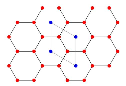
**Fig.** Structure of graphene. Interstitial (blue, the center of hexagon).
