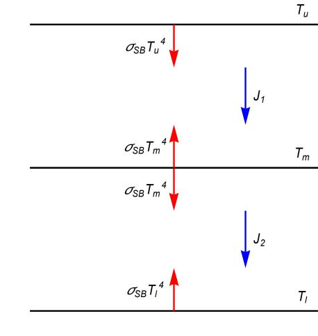
$J_1 = \sigma_{SB}(T_u^4 - T_m^4), \qquad J_2 = \sigma_{SB}(T_m^4 - T_l^4)$
