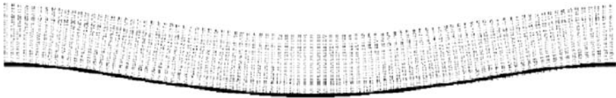
Fig. 24.40. Comparison between MD and beam theory for the deflection of a 20-nm-long fixed-fixed double-walled nanotube (diameter 1.96 nm). The solid black curve is the deflection predicted by beam theory. (Reprinted with permission from Dequesnes et al. [109]. Copyright 2002, Institute of Physics)
