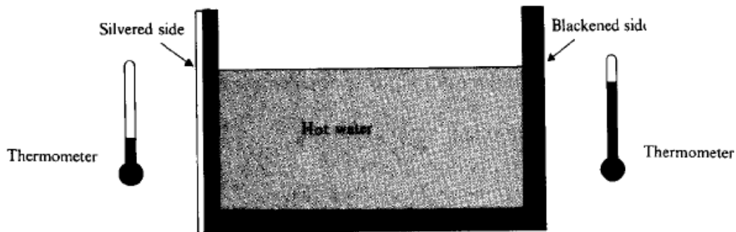
Fig. A classical experiment illustrating Kirchhoff's law. The container is filled with hot water. Its left side is silvered on the outside so that it is a poor absorber. Its right side is blackened so that it is a good absorber. Since the left side is then a poorer emitter of radiation than the right side, the thermometer on the left is found to indicate a lower temperature than the one on the right.
