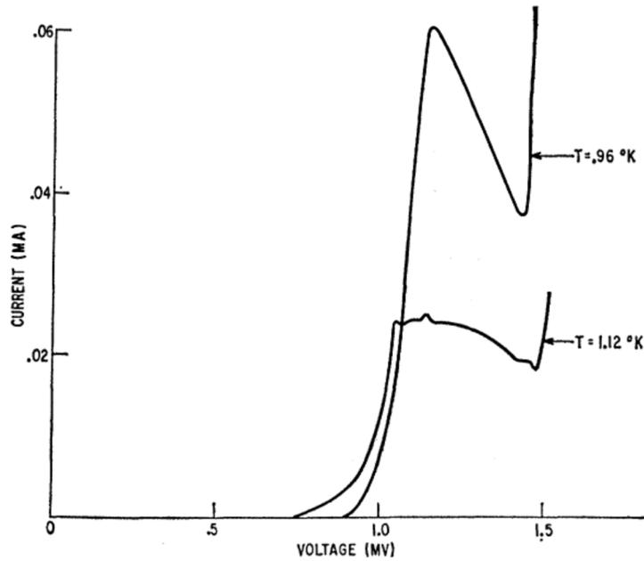
**Fig.** The negative-resistance region traced out for different Al-Al<sub>2</sub>O<sub>3</sub>-Pb sandwiches Fig.17 [I. Giaever and K. Megerle, Phys. Rev. B 122, 1101 (1961)].
