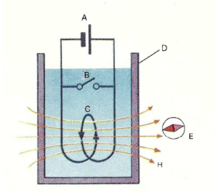
**Fig.** Schematic diagram for the persistent current. *B* is a thermal switch. It is closed so that the current circulates in the superconducting contour inside cryostat *D*, filled with liquid He. *C* is a superconducting ring which generates a magnetic field. The persistent current is used for the generation of an extremely stable magnetic field for the SQUID magnetometer.
