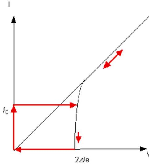
**Fig.** Schematic diagram of quasiparticle  $I$ - $V$  characteristic (usually observed in a S-I-S Josephson *tunneling-type*). Josephson current (up to a maximum value  $I_c$ ) flows at  $V = 0$ .  $\Delta$  is an energy gap of the superconductor. The DC Josephson supercurrent flows under  $V = 0$ . For  $V > 2\Delta/e$  the quasiparticle tunneling current is seen.
