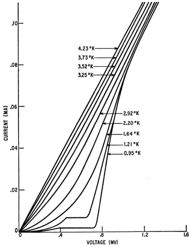
**Fig.**  $I$  vs  $V$  characteristics of an Al-Al<sub>2</sub>O<sub>3</sub>-Sn sandwich at various temperatures. Fig.6 [I. Giaever and K. Megerle, Phys. Rev. B 122, 1101 (1961)].
