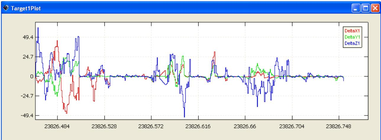
Figure 4. Tracking results of EKF (where DeltaX1, DeltaY1, and DeltaZ1 are the tracking in X-axis, Y-axis, and Z-axis, respectively)
