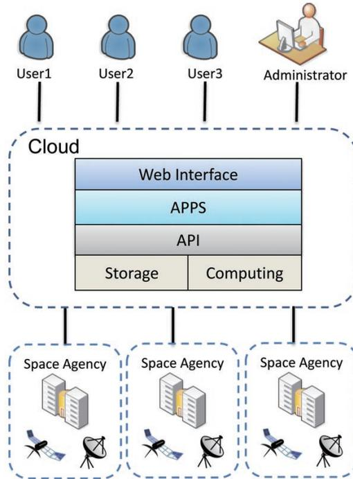
Figure 1. A typical scenario of a Cloud-based SSA system.
