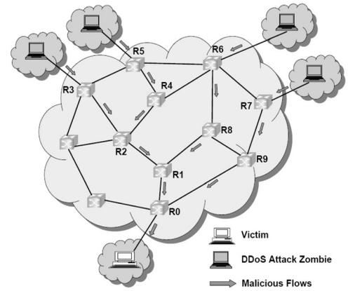
Fig. 1. A traffic superflow by DDoS flooding attacks launched from a large number of zombies toward a common victim host.
