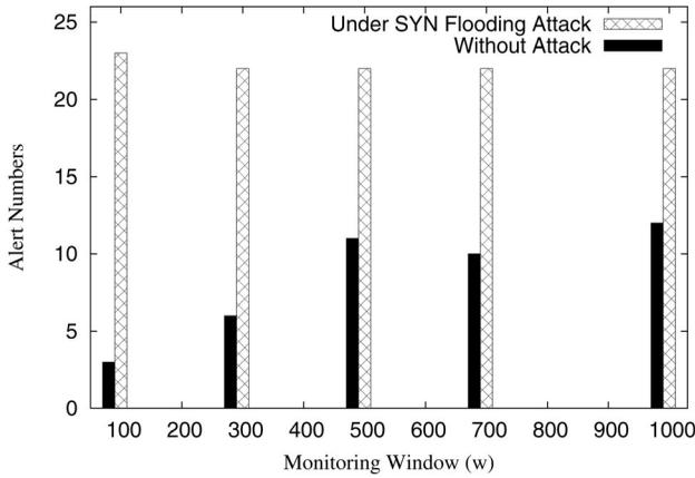
Fig. 12. The router alert number with and without DDoS attacks monitored using various window sizes.
